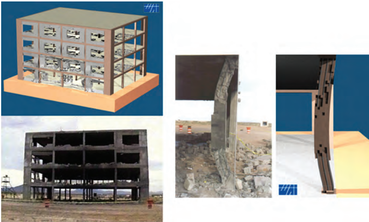
Figure 142: Photos of CTS1 test vs. pretest NLFlex simulation results
