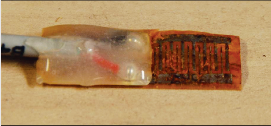
Figure 3-19: Corroded LPR sensor after one-week test
