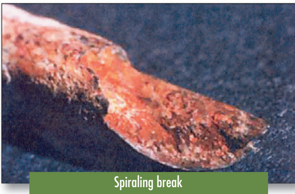
Figure 3-10. Wire breaks and corrosion stages
