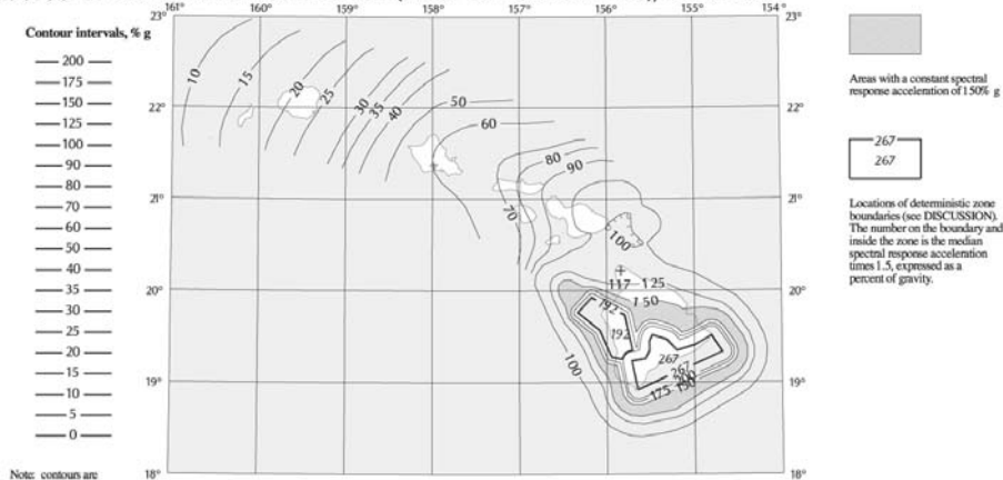
FIGURE 3.3-10 MAXIMUM CONSIDERED EARTHQUAKE GROUND MOTION FOR HAWAII OF 0.2 AND 1.0 SEC SPECTRAL RESPONSE ACCELERATION (5% OF CRITICAL DAMPING), SITE CLASS B
