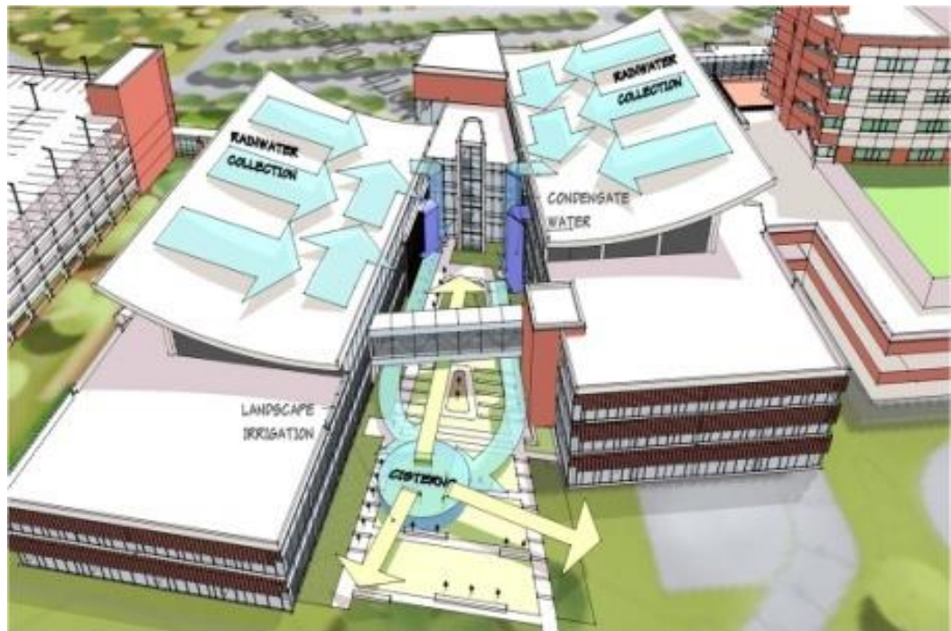
Figure 6. Rainwater capture is integrated into the design of the building as an architectural feature. Swoop roof collect rainwater for diversion into buried cisterns for irrigation use. (Source: HDR)
