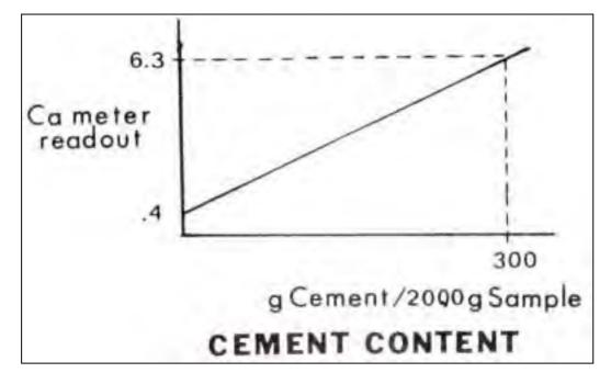
Fig. 5. Calibration Graph for Procedure B
