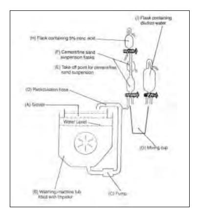
Fig. 2. Equipment for Preparing and Sampling Cement/Fine Sand and Suspension Using Procedure A
