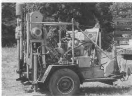
Figure 1. Trailer mounted drill rig
