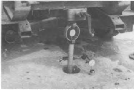
Figure 7. CBR test setup in small aperture
