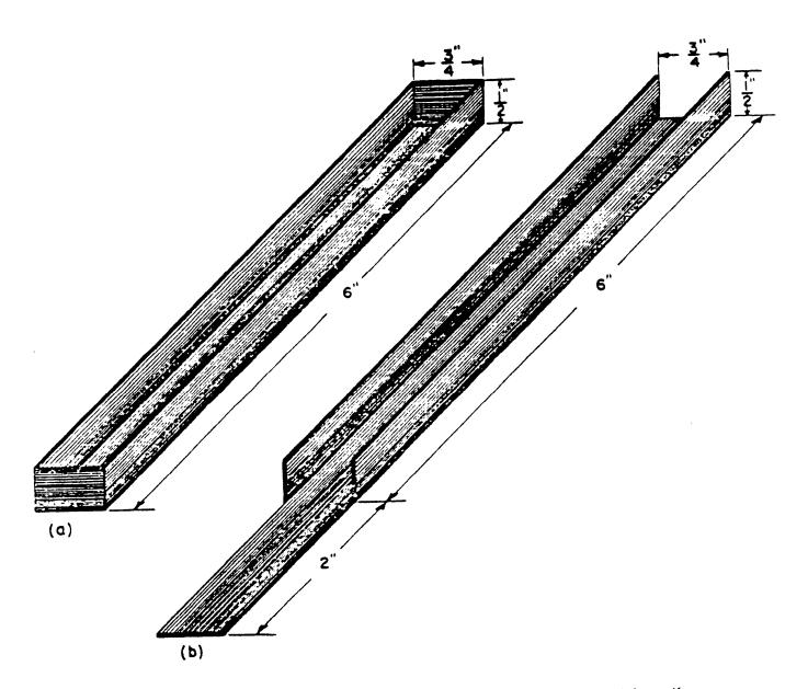
Fig. 1. Channels used for determining rheological properties, (a) for self-leveling or flow type compound ( type ! ), (b) for non-sag type compound ( type 2 )
