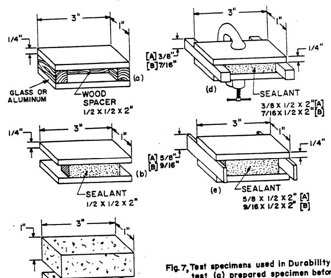
Fig. 7, Test specimens used in Durability test (a) prepared specimen before placement of sealant, (b) Sealant with spacers removed (c) Sealant between mortar blocks, (d) Sealant in the compressed state during heat treatment, (e) Sealant in the extended state.
