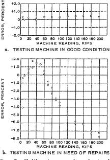
Fig. 2. Calibration results obtained on testing machines
