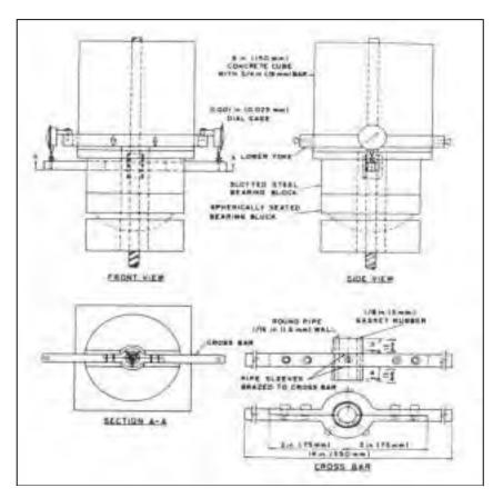
Fig. 2. Measuring and Testing Apparatus for Bond Test
