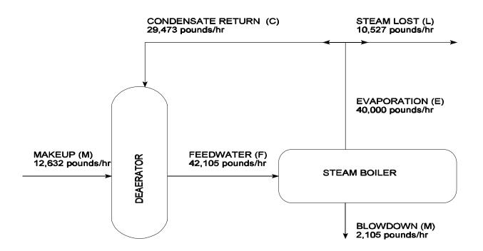
**3-7. Determining chemical treatment** required. Chemical treatment programs involve selecting the type of chemical to be used and establishing a treatment level. These factors are discussed in sections II and III. Blowdown calculations can be used to determine the amount of chemical that needs to be added to meet the treatment objectives.
