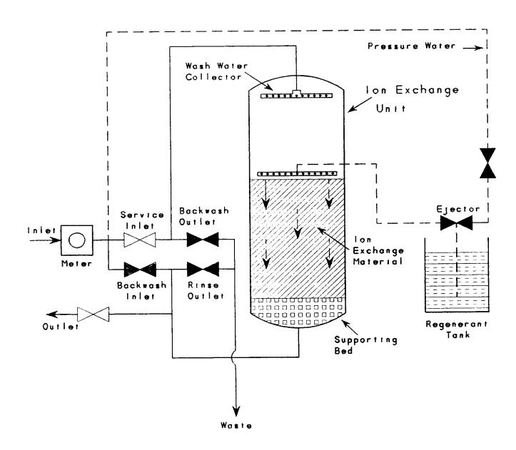
adequate to remove any suspended solids which have been caught on top of the bed. The bed will need to expand by about 50 percent due to the backwash flow rate. The rate should be controlled so that it will not sweep ion exchange material out of the softener into the lines. A backwash rate of 4 to 6 gal/min/ft<sup>2</sup> of bed surface for about 10 minutes is normal, but the manufacturer's recommendations should be followed.
