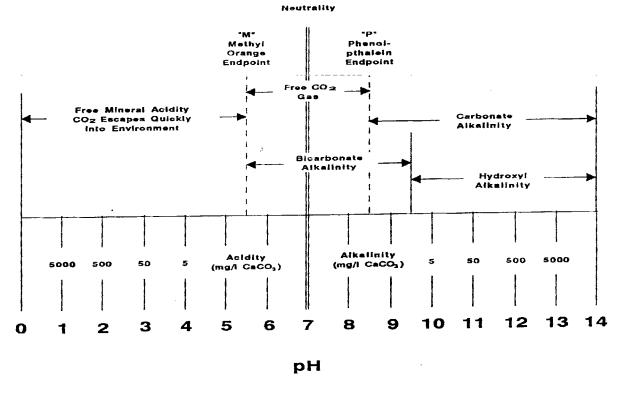
TABLE 6-4 ALKALINITY RELATIONSHIP BASED ON P AND M TESTS
