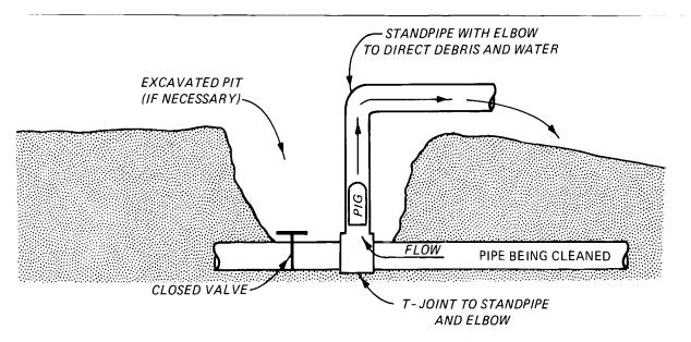
Figure 4. Typical pig retriever configuration.
