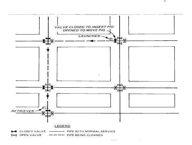
(4) A pressurized water source is necessary for inserting the pig. Pig insertion can be connecting to an upstream hydrant with a backflow preventer in line, or a small water tank 250 gal nation. The pressurized water source will force the pig from the launching joint into the water mair can propel the pig through the line.
