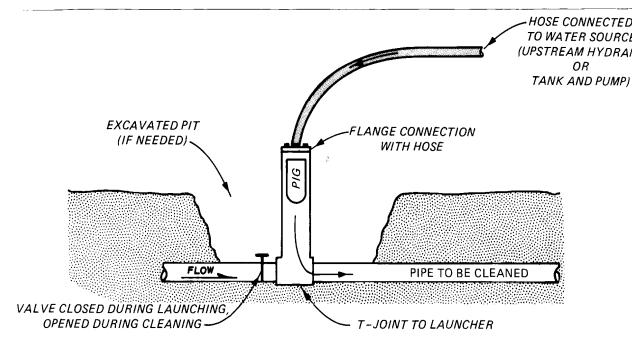
Figure 3. Typical pig launcher configuration.
