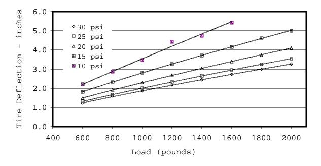
Figure C34. Wrangler tire plunger deflection.
