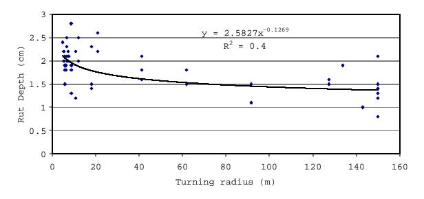
Figure D14. Rut depth of Kevlar tire at low speed.
