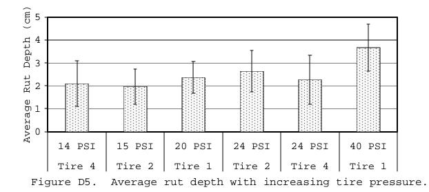
The vehicle spiral tests were designed to compare the field impact of the candidate LEIF tires with regular tires under different dynamic conditions and different field surface conditions. These field tests are required to determine if differences in terrain and vegetative impacts can be observed. The LEIF tires were tested on both a sand test area and two vegetation-covered fields.
