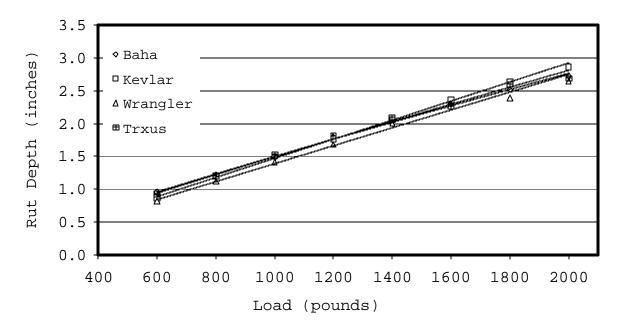
Figure C26. Rut depth at 10 psi.
