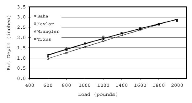
Figure C29. Rut depth at 25 psi.
