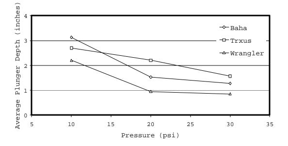
Figure D2. Plunger depth for each tire.Rutting Field Tests
