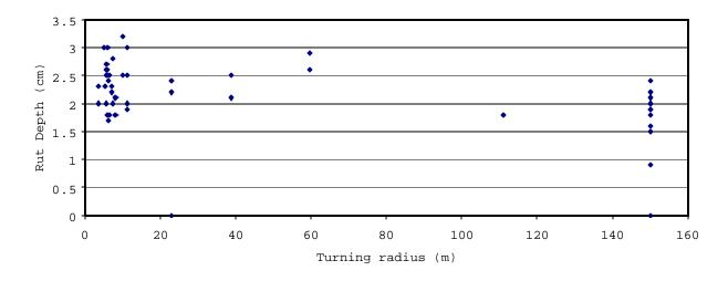
Figure D15. Rut depth of Goodyear tire at low speed.
