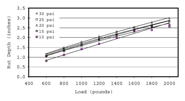
Figure C24. Wrangler tire rut depth.
