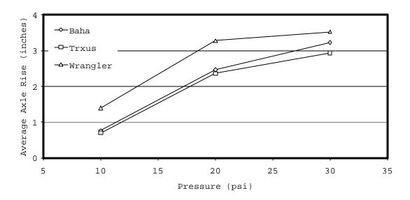
Figure D1. Axle rise for each tire.
