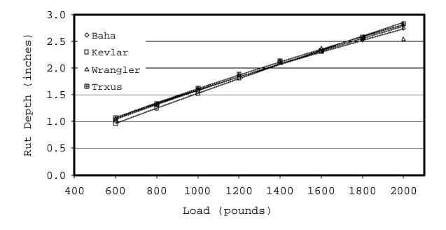
Figure C27. Rut depth at 15 psi.
