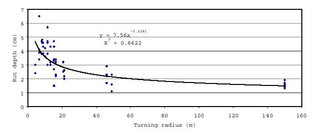
Figure D16. Rut depth of Kevlar tire at high speed.
