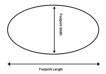
Figure C2. Diagram of measured tire footprint area.
