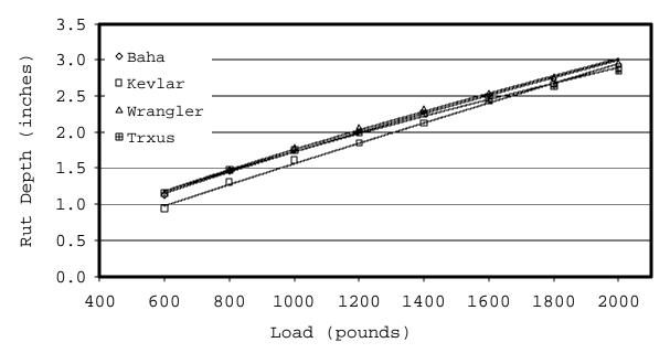
Figure C30. Rut depth at 30 psi.
