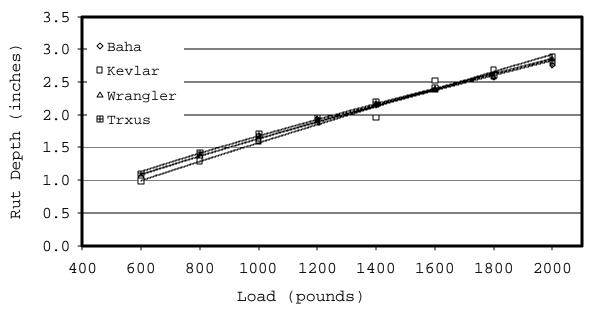
Figure C28. Rut depth at 20 psi.
