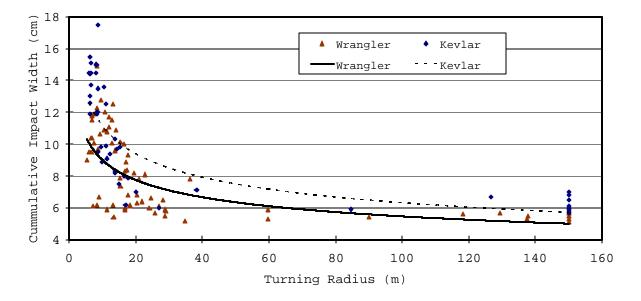
Figure D24. Tire impact comparison.
