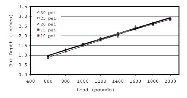
Figure C23. Kevlar tire rut depth.
