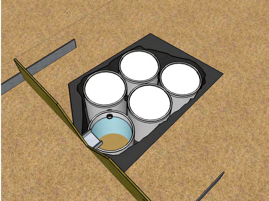
Figure B-2. Plot runoff collection structure.
