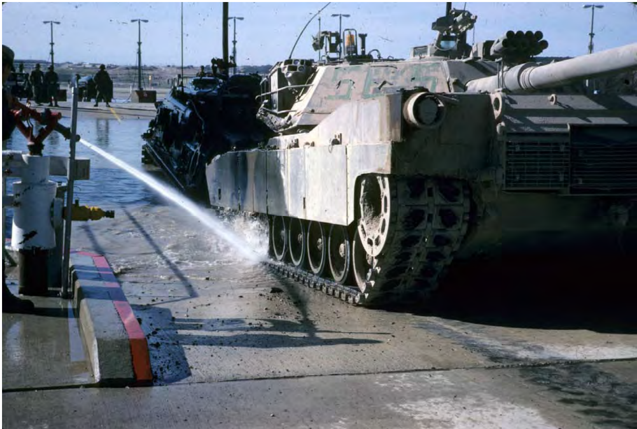
Figure A-11. An M-1 tank being towed through a bath (photo by ERDC-CERL).
