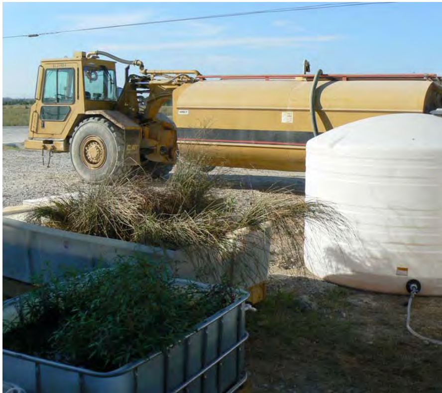
Figure A-1. Leachate transport vehicle.
