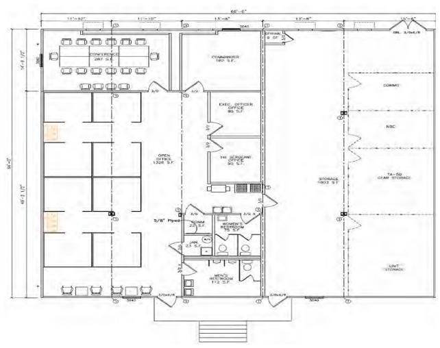
Figure B-3. Example of a typical full-complement company facility.
