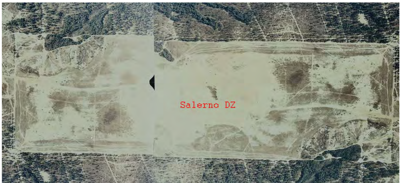
Figure C-3. Salerno DZ in December 1995 before restoration, showing the normal practice of keeping the drop zone free of all woody and grassed vegetation, which resulted in severe erosion and degradation.
