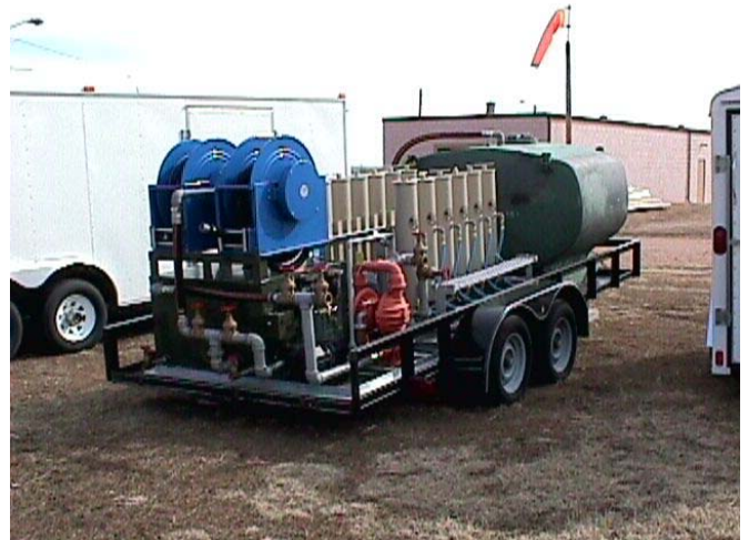
Fuel Filtration Unit Mounted on a Tandem Axle Transportation Trailer
