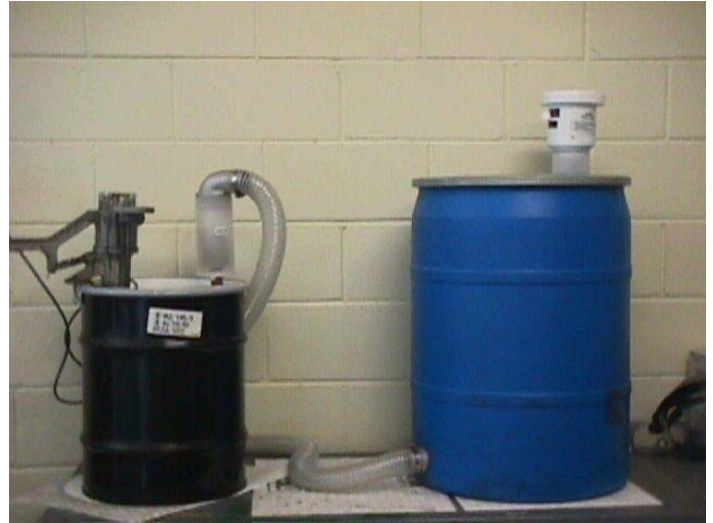
Aerosol Can Puncturing Apparatus and Activated Carbon Filter
