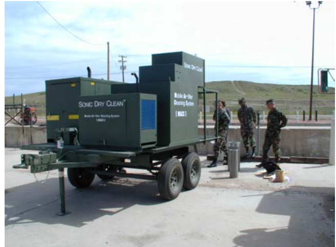
Air Filter Cleaning Unit Mounted on a Tandem Axle Transportation Trailer
