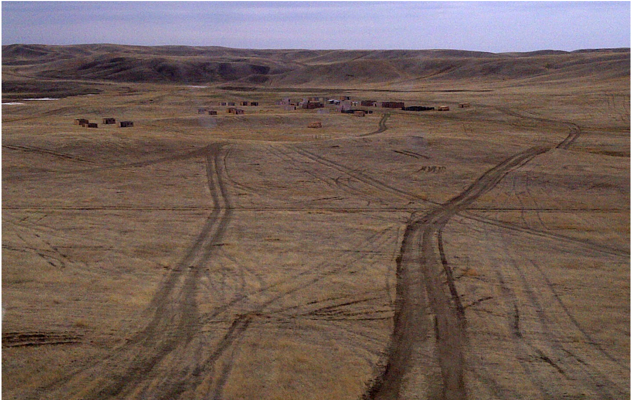
Figure D-7. This panoramic view of a Canadian MOUT site shows the impact of various trafficking patterns and array of vehicular approaches (ERDC-CERL, 2014).
