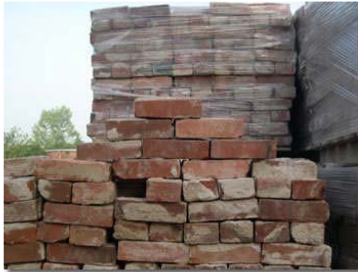
Figure D-6. Pallets of salvaged bricks.
