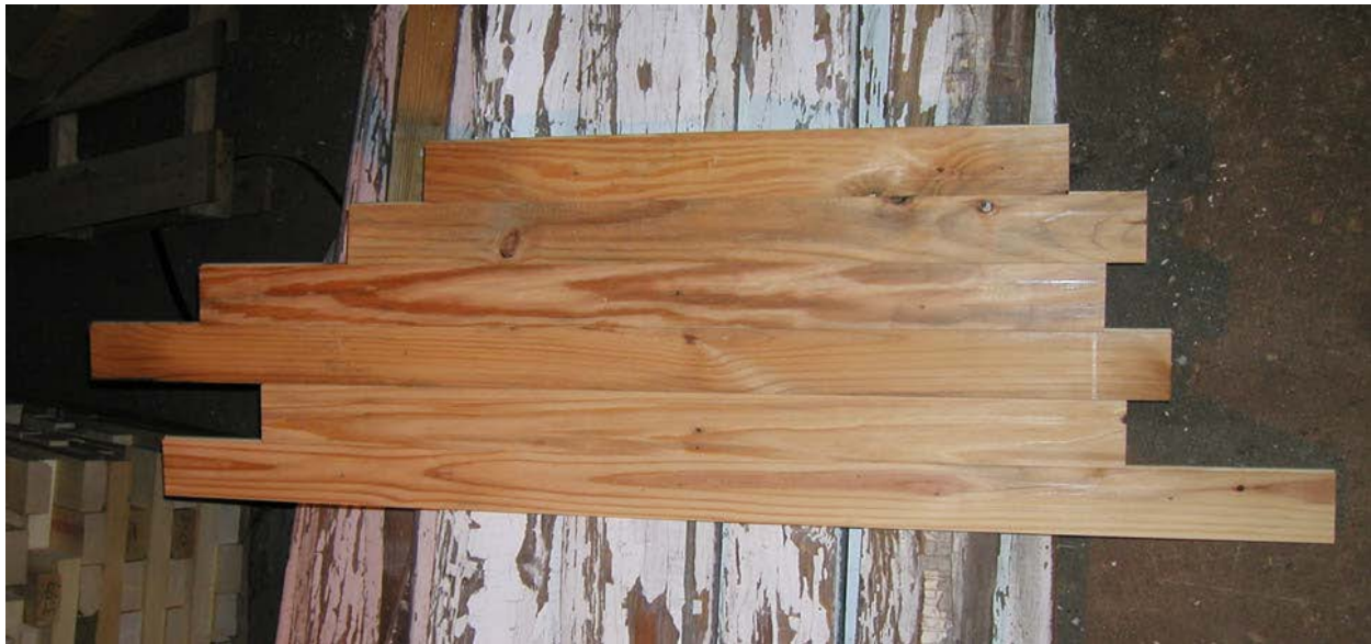
Figure D-5. Tongue-and-groove flooring (foreground) reclaimed from painted wood siding (background).
