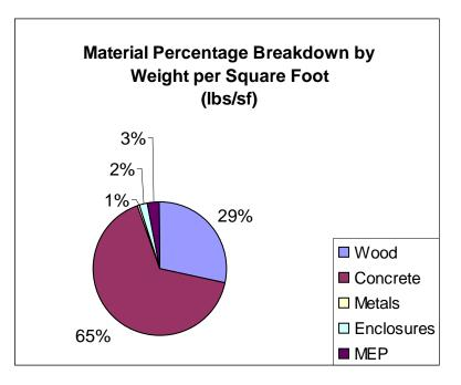
Figure B-7. Summary weight and percentage of recyclable or salvageable material categories from a typical light-framed housing unit, as calculated in Table B-1.
