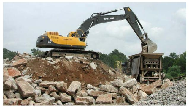
Figure C-1. Concrete recycling with on-site crusher.
