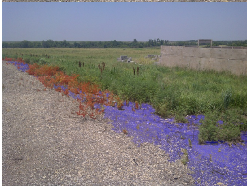
7 Figure C-5. Herbicide-treated gravel pad (unaltered view on top). The altered 8 bottom image shows bare soil in purple, with vegetation death shown in red 9 (ERDC-CERL).
