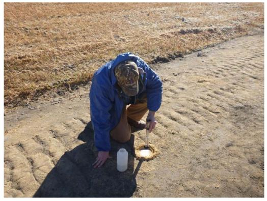
Figure B-6. Bioswale infiltration testing.
