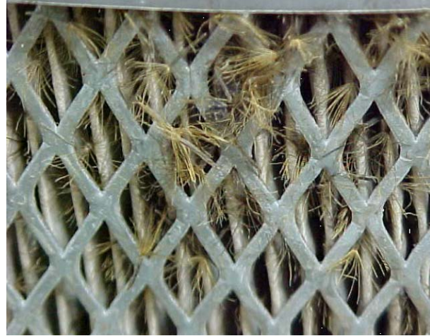
Figure A2. Siam weed ( Chromolaena odorata ) in cooling system of a military armored personnel carrier after washing (photo by Stuart Henson, AQIS).
