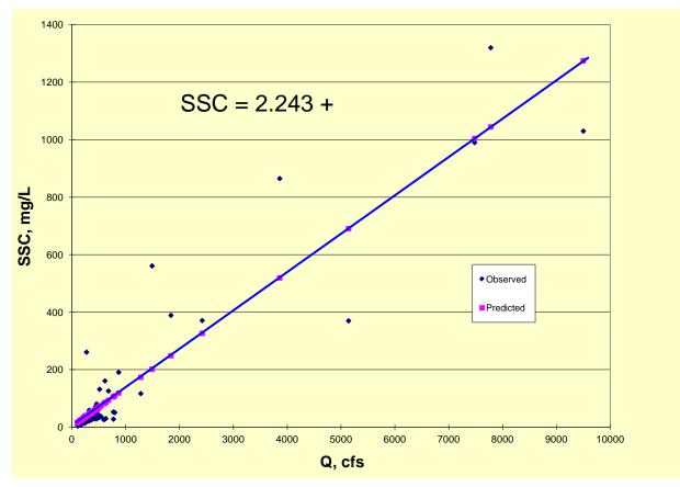
Figure D-2. Regression results depicting relationship between flow and suspended-sediment concentration.
