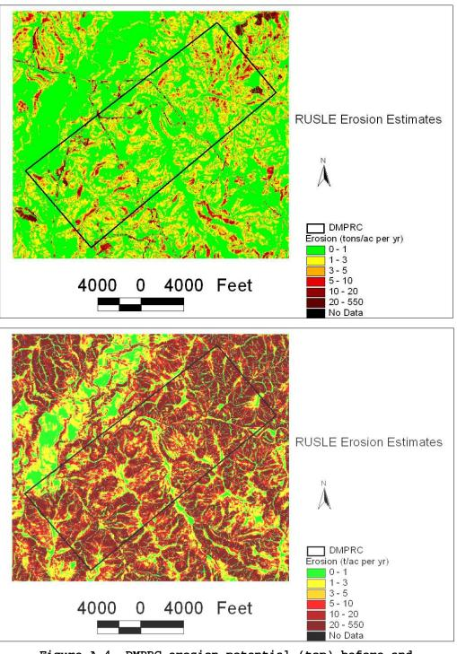
Figure A-4. DMPRC erosion potential (top) before and after construction (bottom).1
