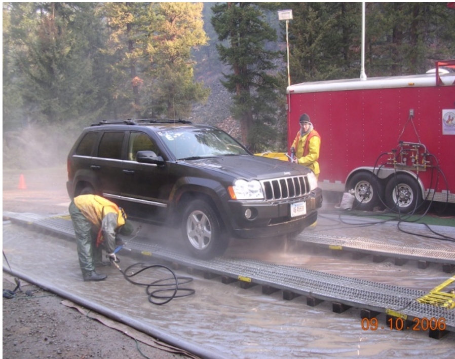
Figure A-1. A relocatable vehicle washing system.
