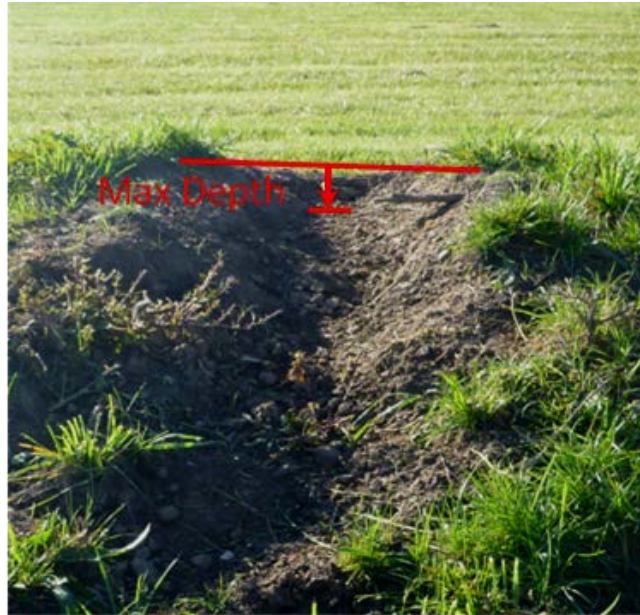
Figure B-12. Schematic of maximum depth measurement used to quantify treatment success at Camp Atterbury demonstration site (ERDC-CERL 2012).
