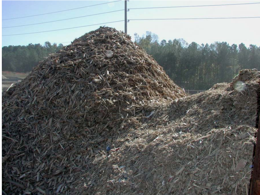
Figure A-8. Lumber debris shredded for boiler fuel.
