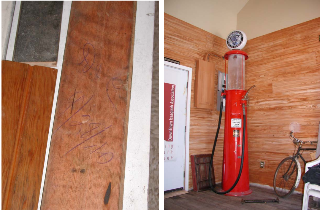
Figure A-28. Custom-grade Douglas Fir siding from Fort Lewis (left), used for historic building restoration near Seattle.
