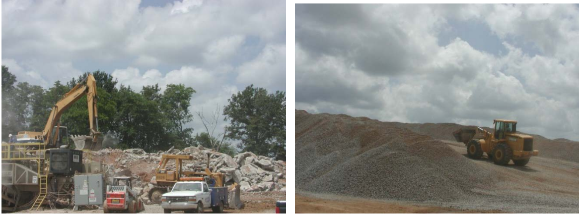
Figure A-21. Contractor's concrete recycling operation and recycled concrete aggregate product adjacent to Fort Campbell.
