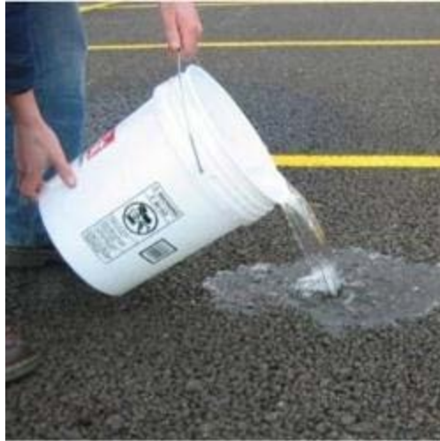
Figure H-45. Presentation of how well the porous asphalt allows water to percolate through the pavement (City of Sturgis 2011).
