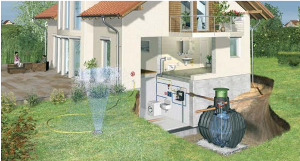
Figure H-18. Example diagram of an underground plastic cistern shown, as would be connected to a house rainwater and greywater system (GRAF 2011).
