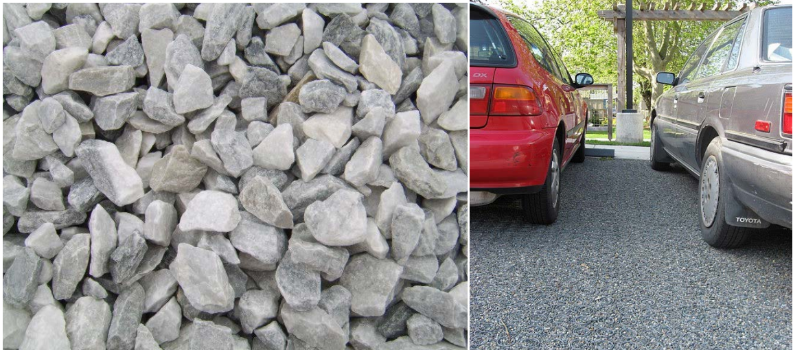
Figure H-72. Left: Close up of crushed stone - note the angular edges (Nashville Stone n.d.); Right: Pervious parking next to a pocket park in Seattle (EPA 2007).
