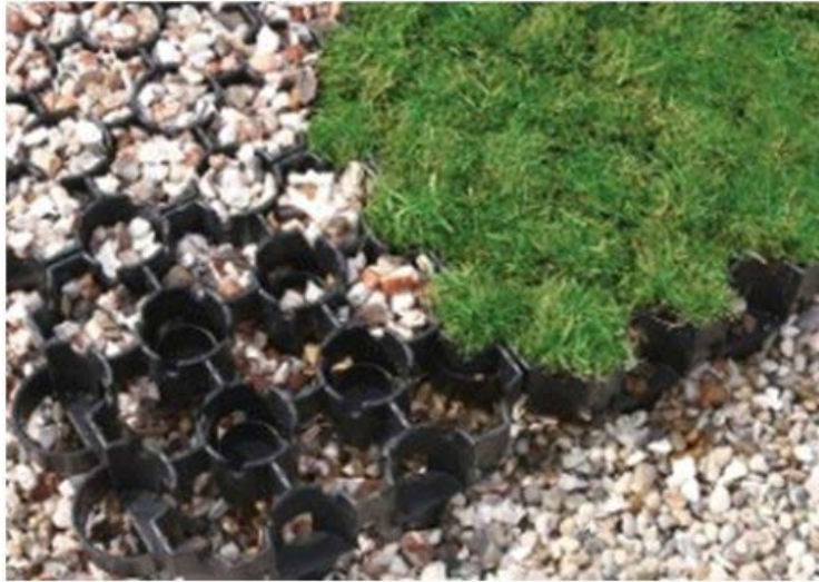
Figure H-47. One example of cellular plastic that shows the stages of installation with some cells empty, some filled with gravel growing media, and some fully grown-in with grass (Boddingtons 2011).
