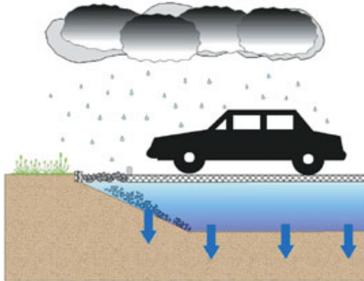
Figure H-54. Diagram of a typical recharge bed under a porous parking lot (Adams, 2003).
