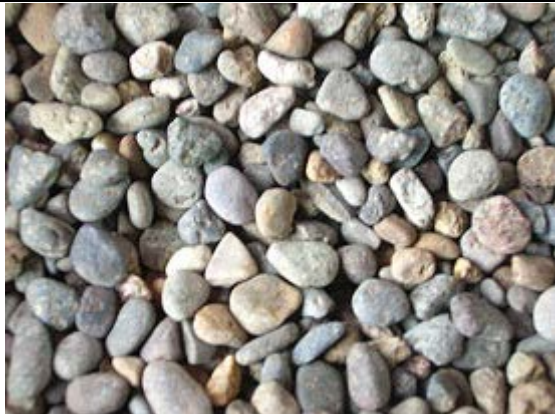
Figure H-75. Close-up of pea gravel -- note rounded edges (Bark Boys Inc. 2009).
