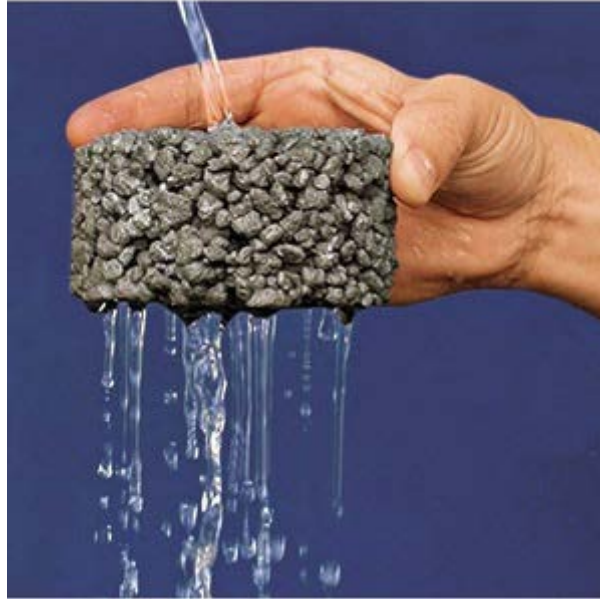
Figure H-46. Example of porous concrete water flow (VDC Green 2010).
