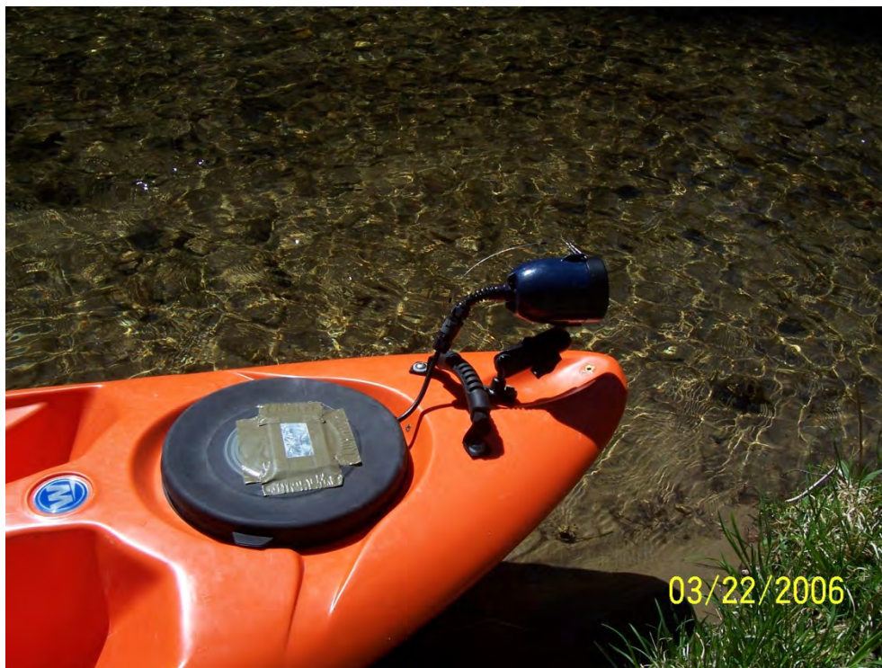
Figure A-2. The Splashcam Deep Blue video camera, mounted to the kayak bow to acquire above-water footage
