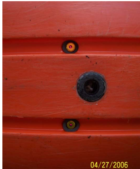
Figure A-3. A flush-mounted camera (middle) and two parallel laser pointers (top and bottom) on the kayak hull.
