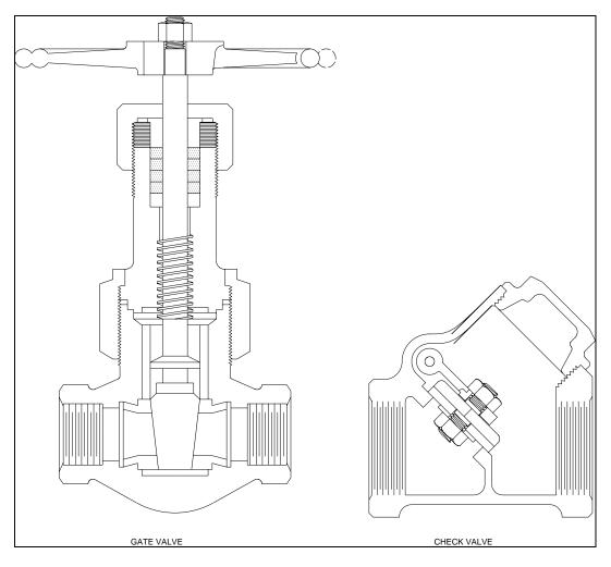
Figure 23-6. Gate valve and swing check valve
