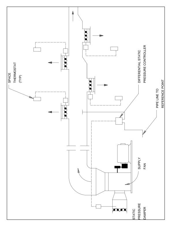
Figure 19-6. Typical air handling systems controls
