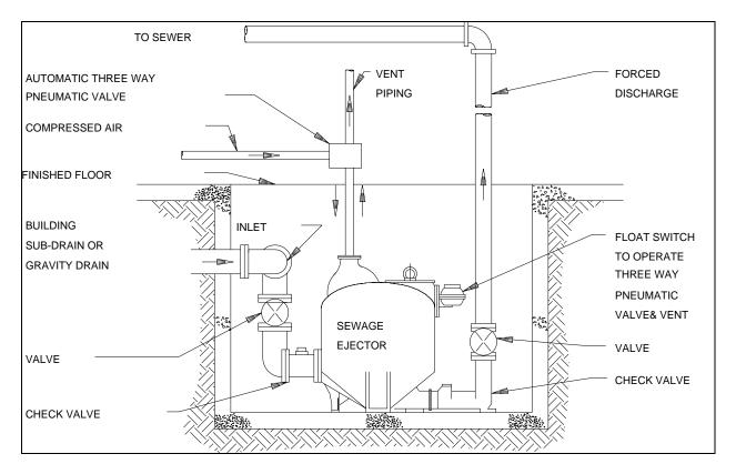
Figure 23-5. Pneumatic sewage ejector
