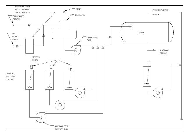
Figure 18-4. Typical steam boiler installation
