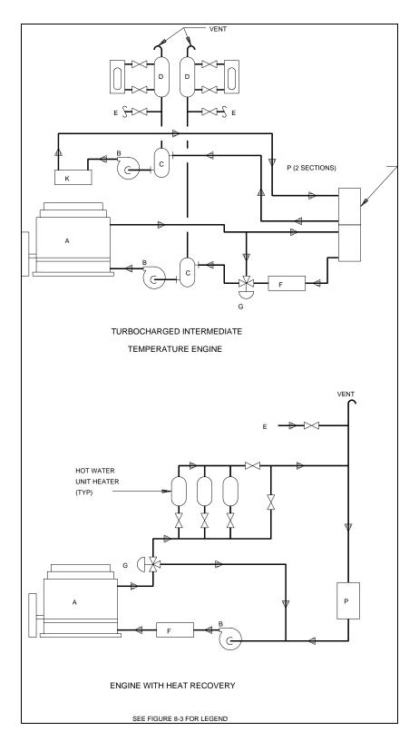
Figure 13-2. Examples of engine cooling systems (2)
