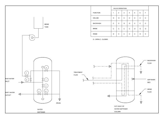
Figure 18-5. Basic water softener system
