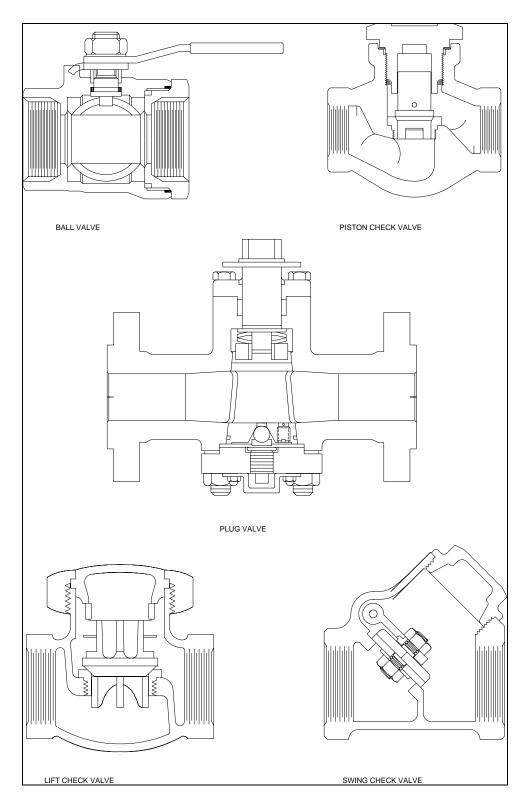
Figure 16-3. Typical valves used in water service (2)
