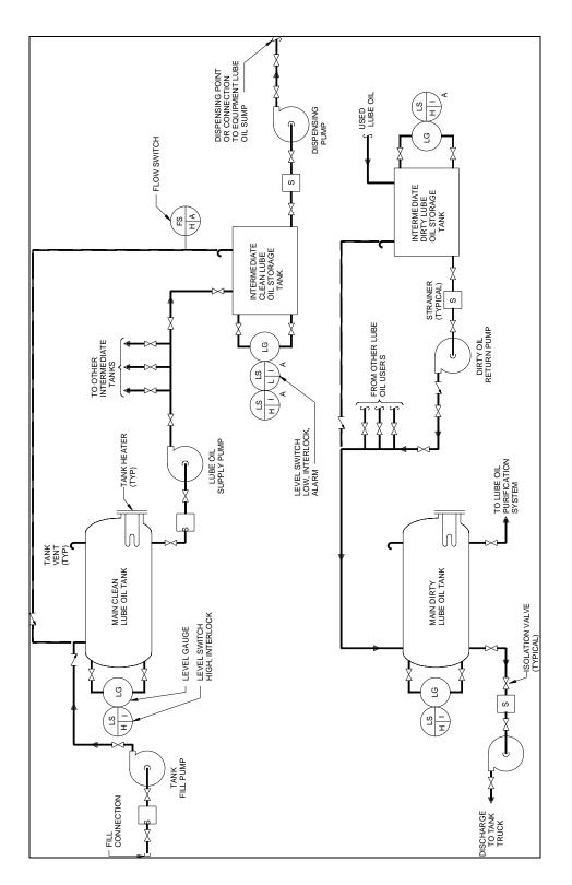
Figure 11-2. General lube oil storage and dispensing system
