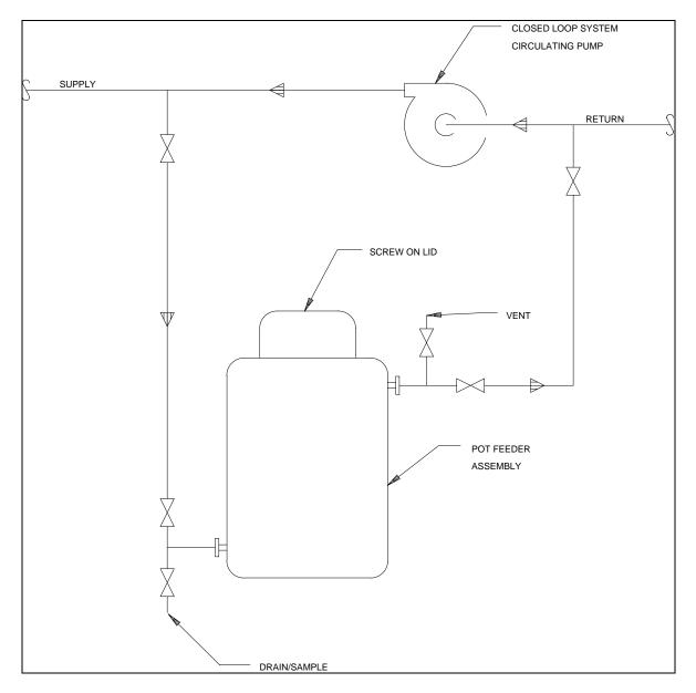
Figure 18-2. Typical pot feeder bypass installation
