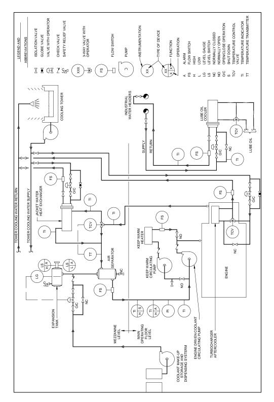
Figure 13-4. Typical primary service diesel engine cooling system
