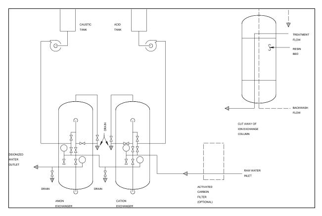
Figure 18-6. Basic ion exchange unit
