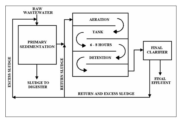
Figure 23-2. Conventional plug flow activated sludge flow diagram
