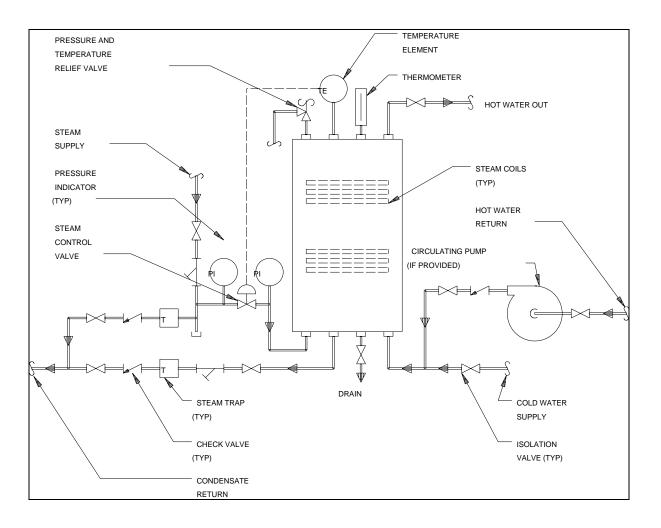
Figure 17-5. Semi-instantaneous steam water heater
