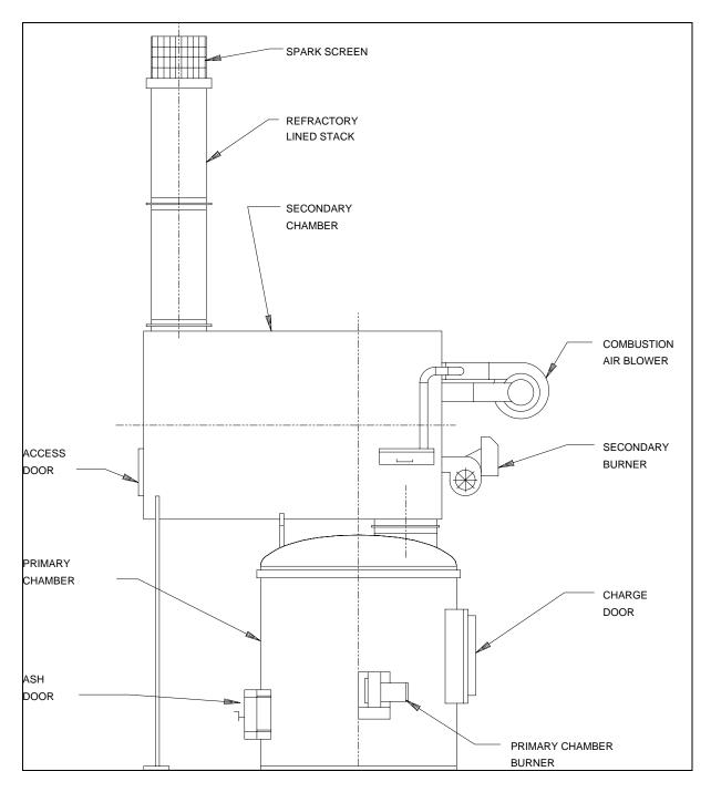
Figure 15-1. Vertical dual chamber incinerator
