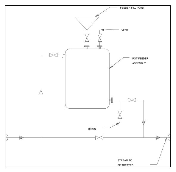
Figure 18-1. Typical fill system pot feeder installation
