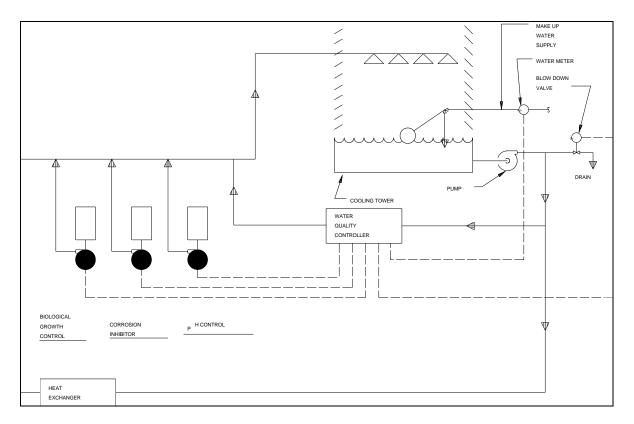
Figure 18-3. Open-loop chemical treatment system
