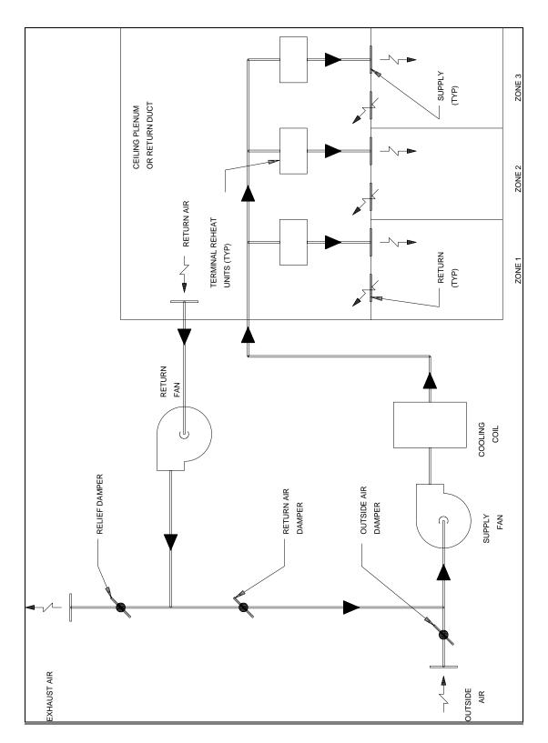
Figure 19-4. Air handling system with reheat
