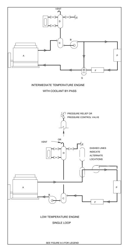
Figure 13-1. Examples of engine cooling systems (1)
