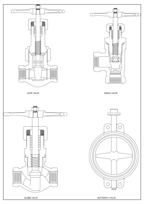
Figure 16-2. Typical valves used in water service (1)
