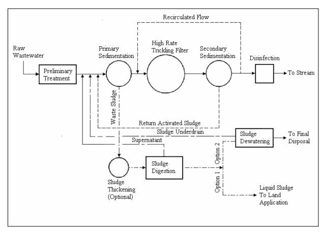
Figure 23-1. Typical trickling filter process treatment train
