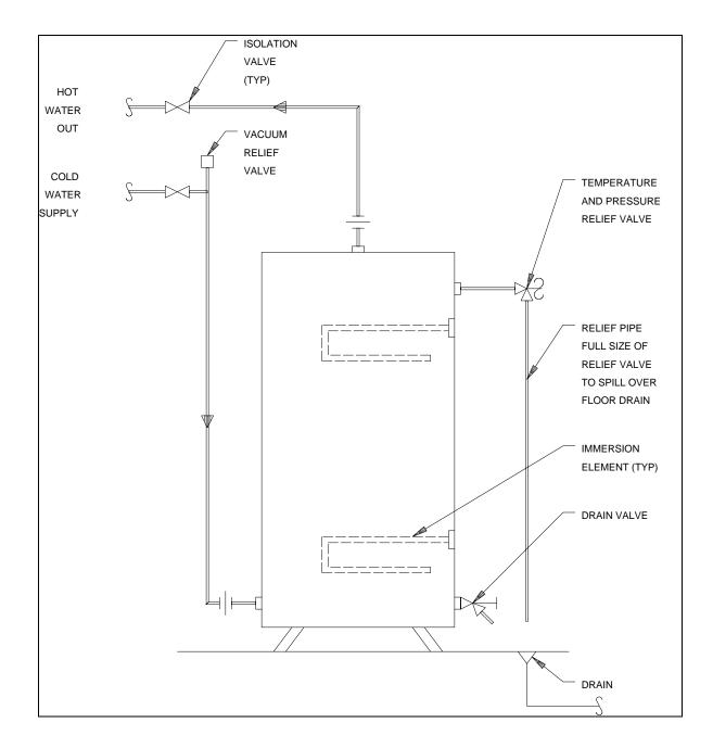
Figure 17-3. Electric water heater
