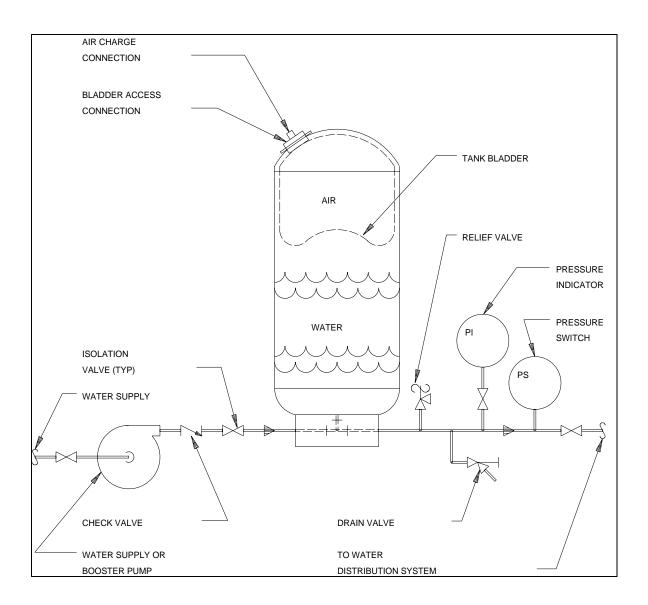
Figure 17-2. Bladder tank installation
