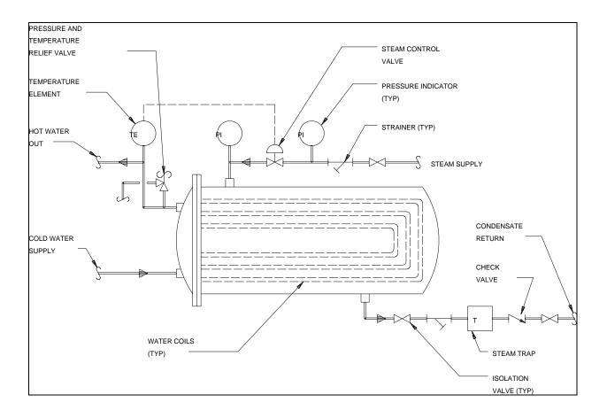
Figure 17-4. Instantaneous steam water heater
