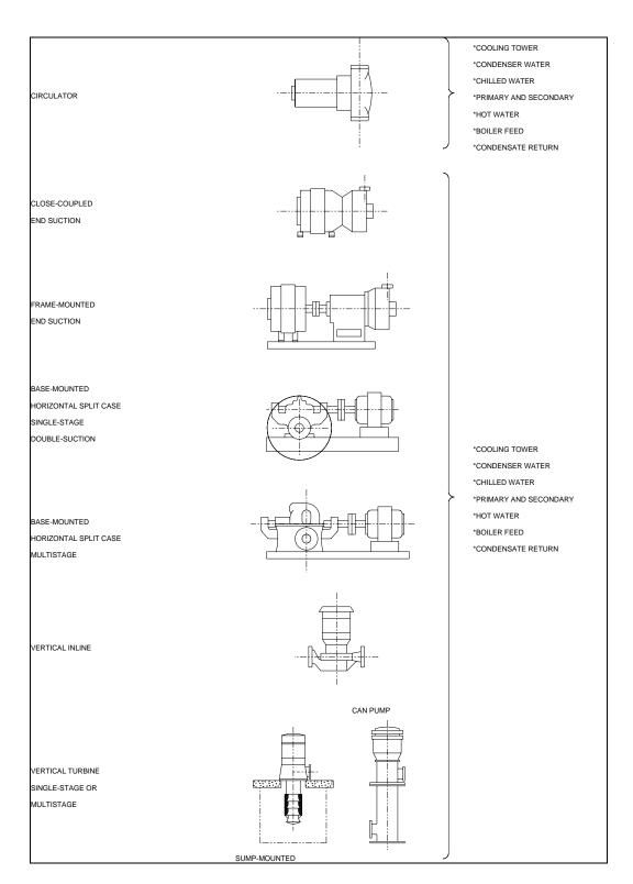
Figure 16-1. Variations of centrifugal pumps
