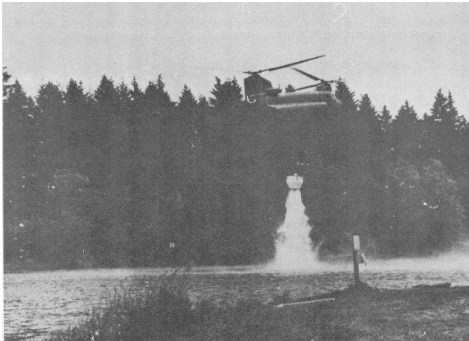
Figure 10-16. Testing water bucket of chinook helicopter.
