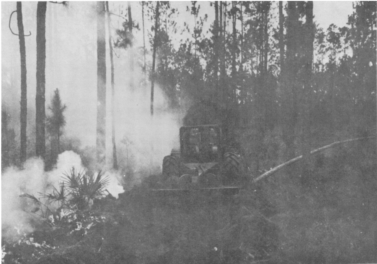
Figure 10-11. Fire-line construction using heavy fire-line plow.
