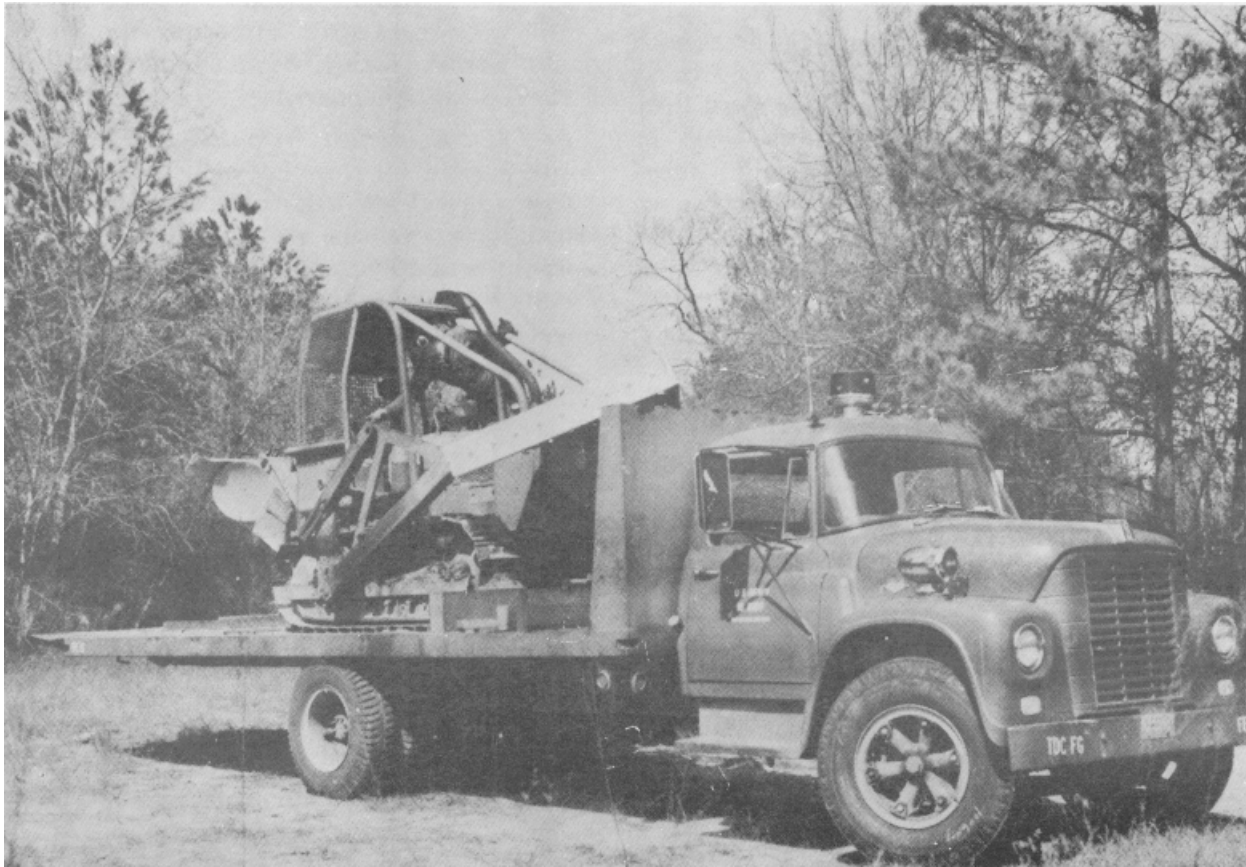
Figure 10-14. Fire-fighting equipment on transport truck with roll-back ramp.
