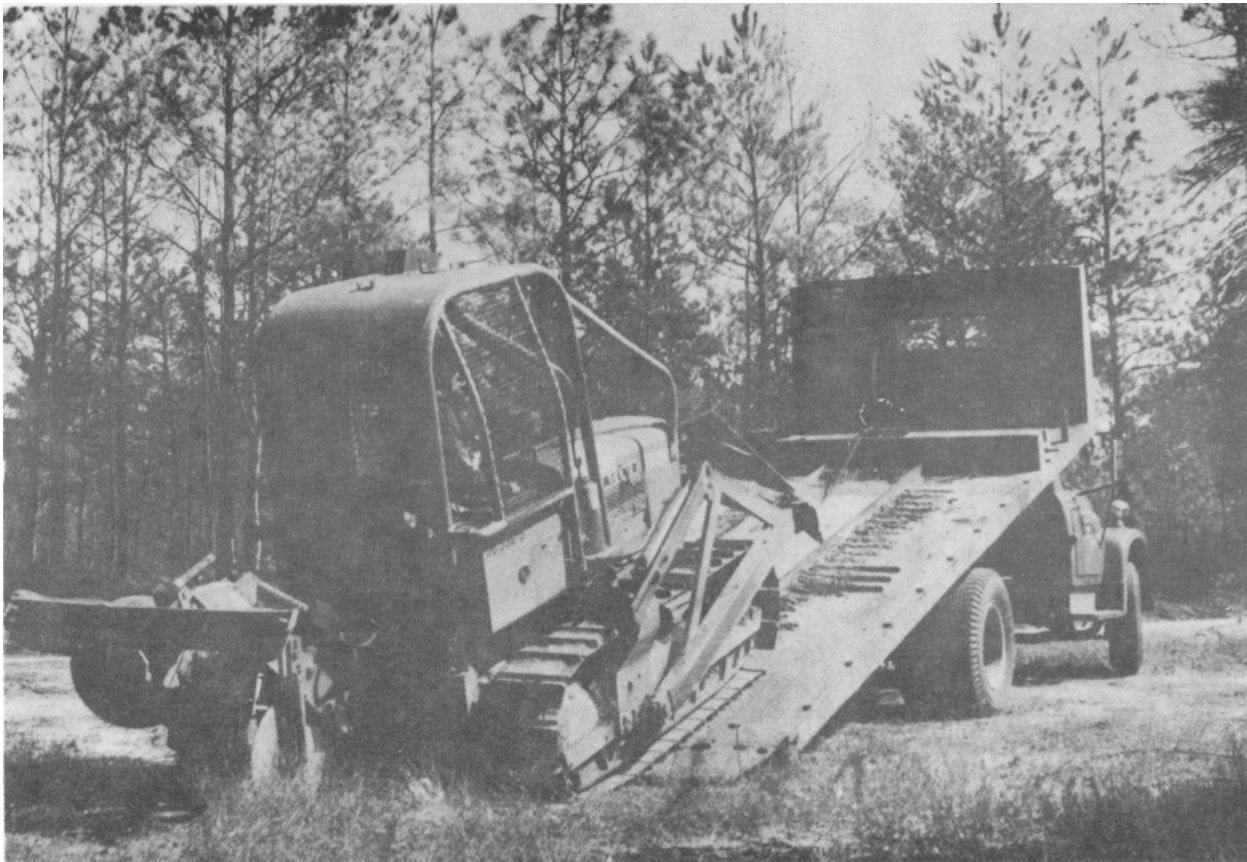
Figure 10-13 Loading a light tractor with fire plow attached
