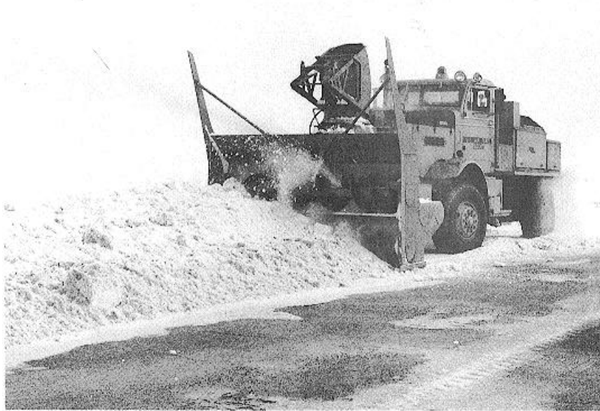
Figure 9-2. Two-element rotary plow with twin horizontal-axis helical augers.
