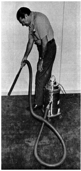
Figure E-7. Wet/dry tank vacuum.
