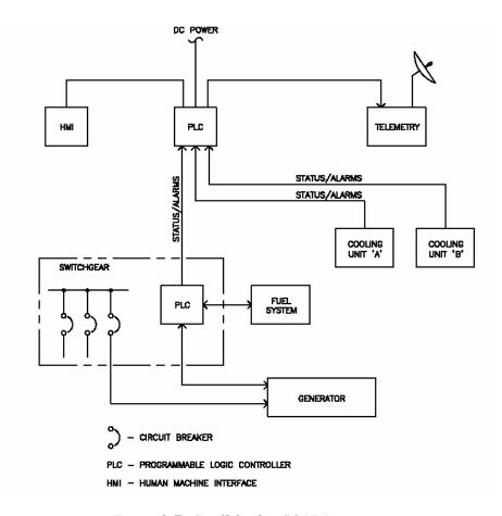
Figure 3-7. Small facility SCADA system
