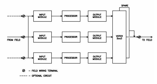
Figure 3-6. Triple-redundant PLC configuration
