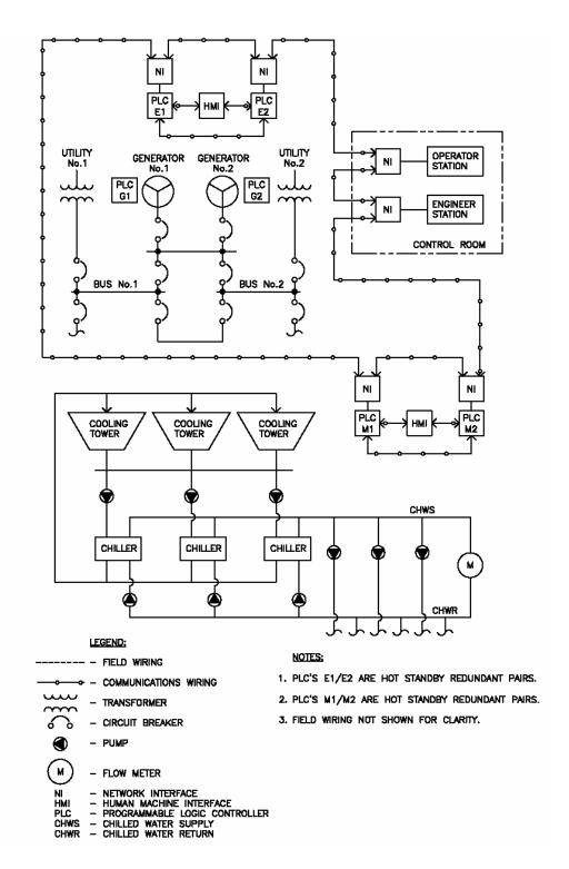
Figure 3-9. Medium facility SCADA system – redundant M/E components
