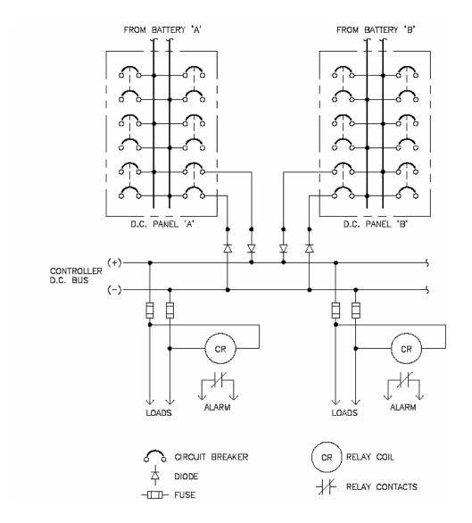
Figure 5-3. Diode-based "best-battery" selector circuit
