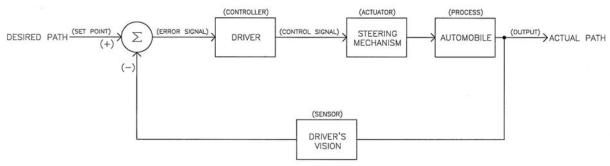
Figure 2-2. Analog control system block diagram
