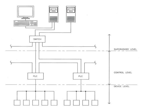
Figure 4-1. Typical SCADA network levels
