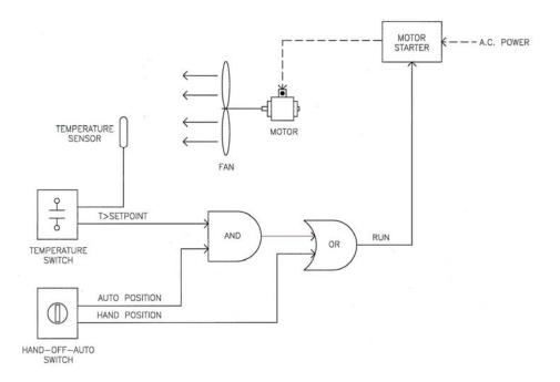
Figure 2-1. Discrete control system block diagram
