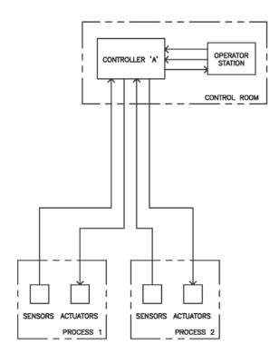
Figure 3-2. Centralized control system architecture
