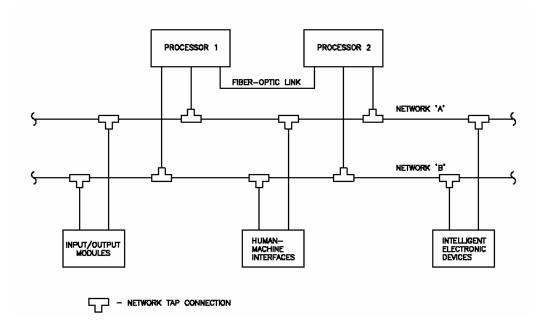
Figure 3-5. Typical redundant PLC configuration
