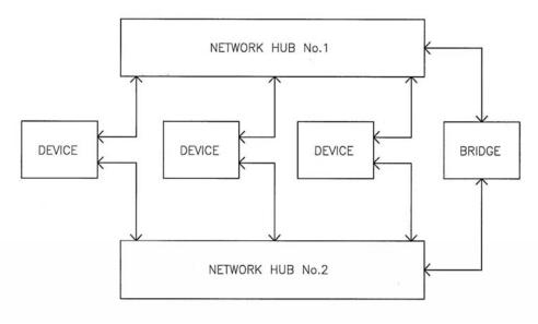
Figure 4-5. Fully redundant network
