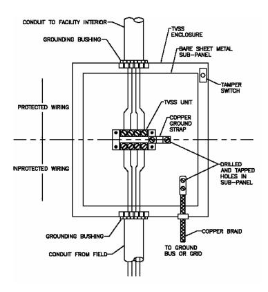
Figure 7-1. Signal level TVSS installation
