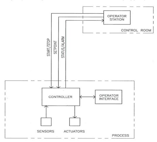
Figure 3-1. Local control system architecture
