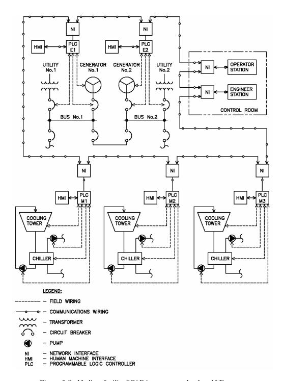
Figure 3-8. Medium facility SCADA system – redundant M/E systems
