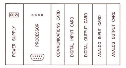
Figure 3-4. Typical PLC rack
