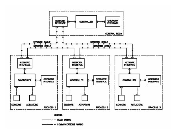
Figure 3-3. Distributed control system architecture
