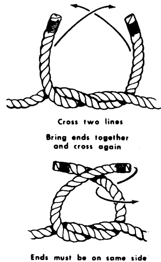
Figure 2-46. Tool hoisting hitch.
