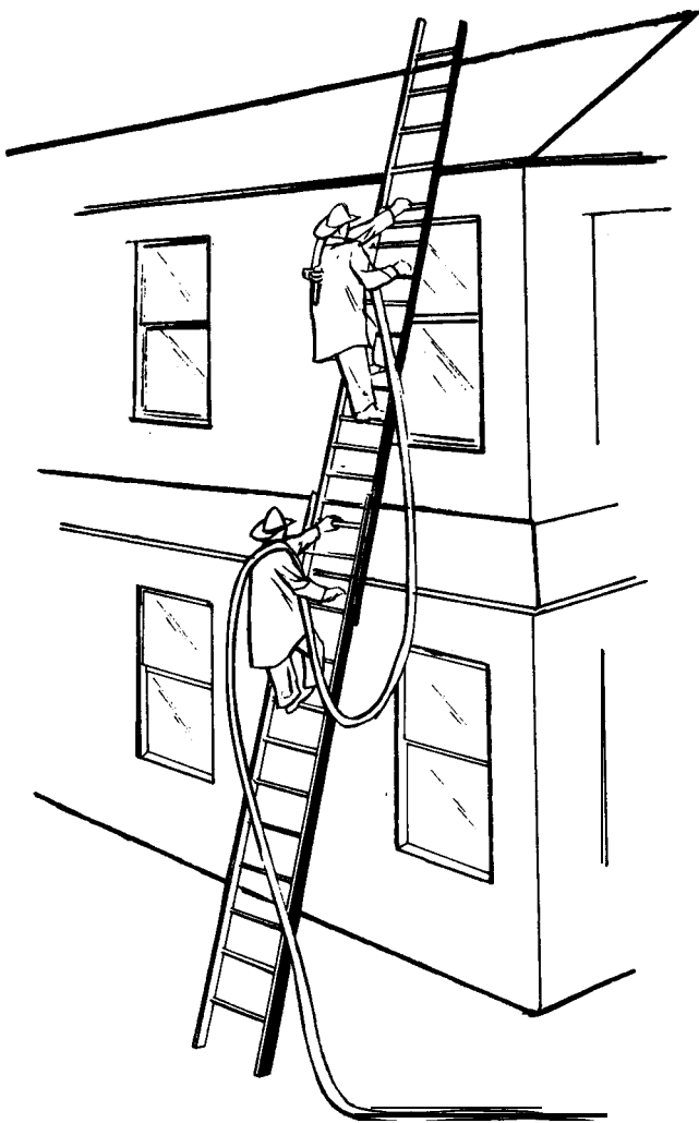
Figure 4-24. Advancing a hose up a ladder.
