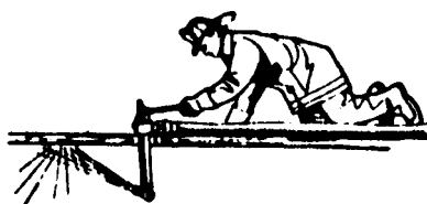
CELLAR PIPE IN OPERATION
