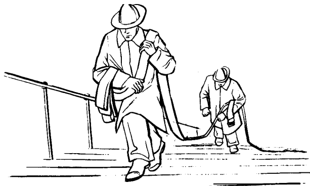
Figure 4-25. Advancing a hose up a stairway.
