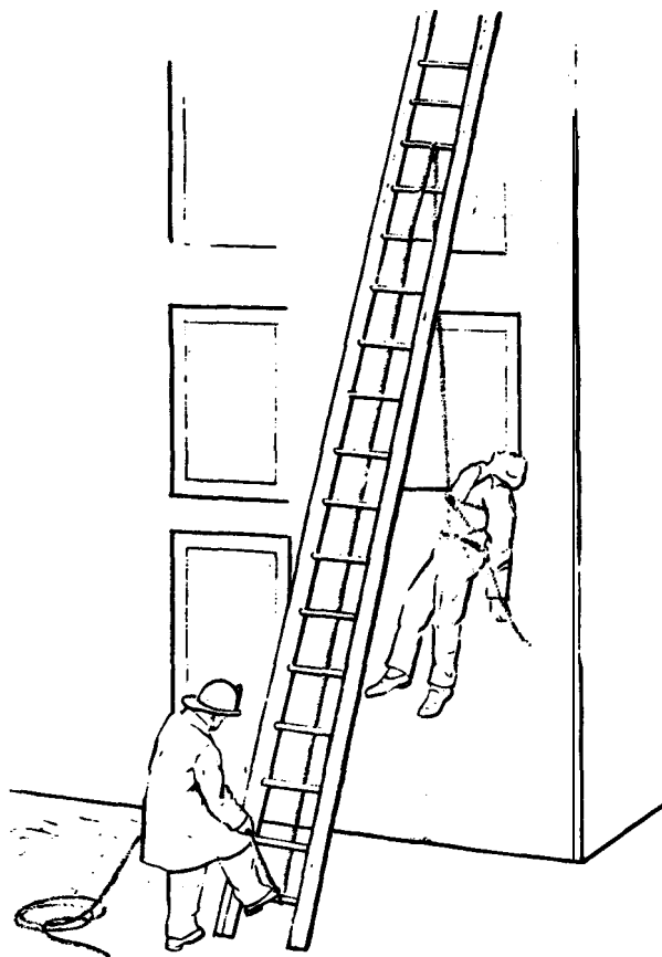
Figure 4-80. Lowering victim with rope and ladder.
