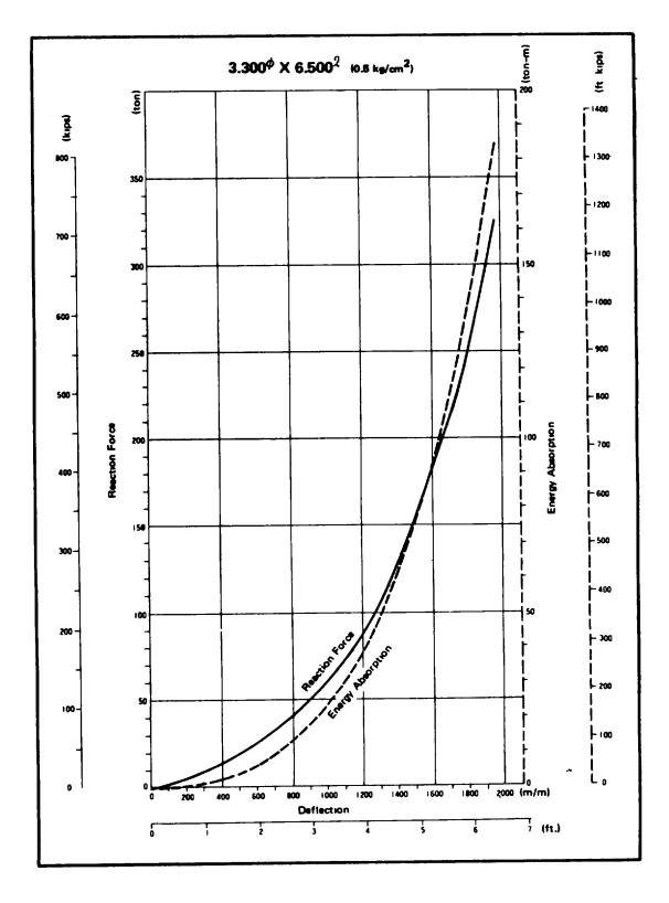
Figure 9-18. Yokohama Pneumatic Rubber Fenders (this size used for berthing 25,000- to 200,000 ton ship).
