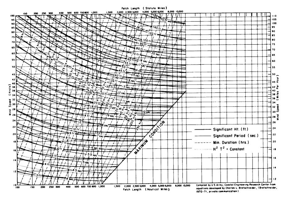
Figure 5-3. Deepwater wave forecasting curves (for fetches of 100 to more than 1,000 miles)
