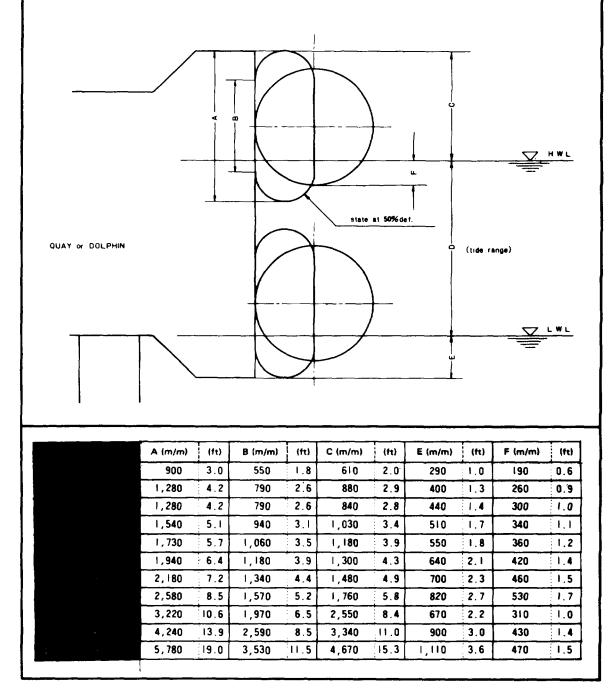
Figure 9-16. Yokohama Pneumatic Rubber Fenders (dimension of jetty at the time of installation).
