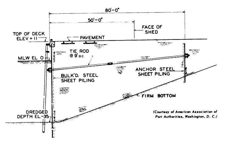
Figure 8-11. Solid fill-type wharf construction with steel sheet pile bulkhead.
