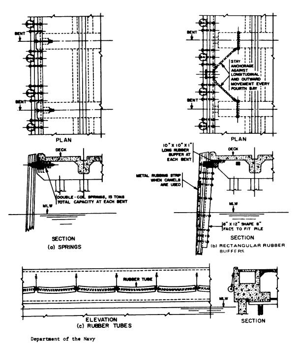
Figure 9-5. Resilient Fender System (spring rubber bumper).
