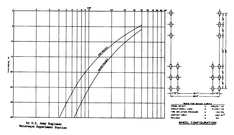
Figure B-21. Flexible Pavement Design Cure for P&H 6250- TC(mobile crane).
