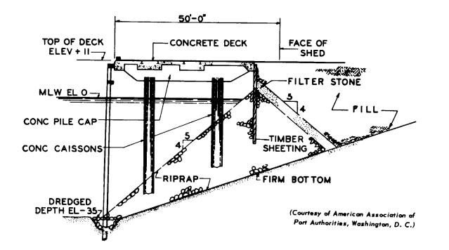
Figure 8-8. High-Level Open-Type Wharf Construction with Concrete Deck on Precast Prestressed Concrete Caissons.
