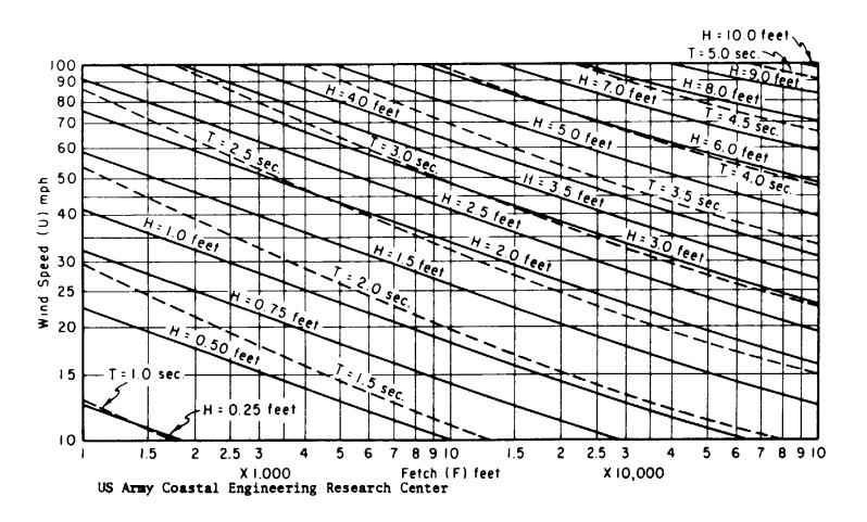
Figure 5-9. Forecasting curves for shallow-water waves (constant depth = 30 feet).
