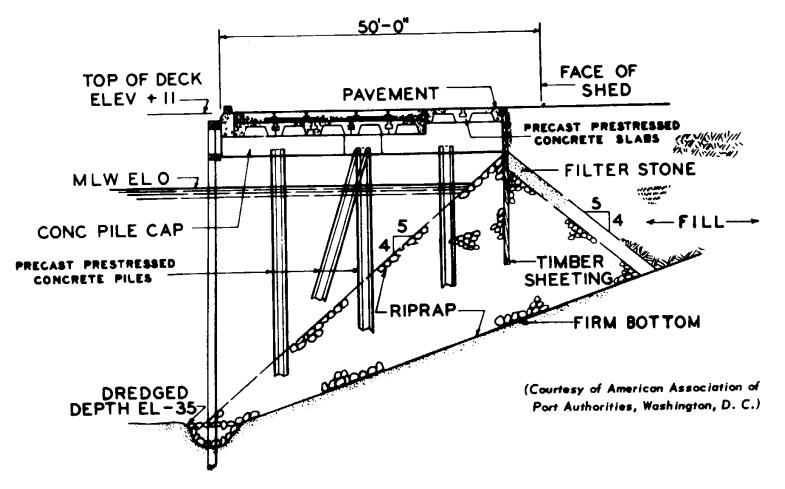
Figure 8-9. High-Level Open-Type Wharf Construction with Precast Concrete Deck on Concrete Piles.
