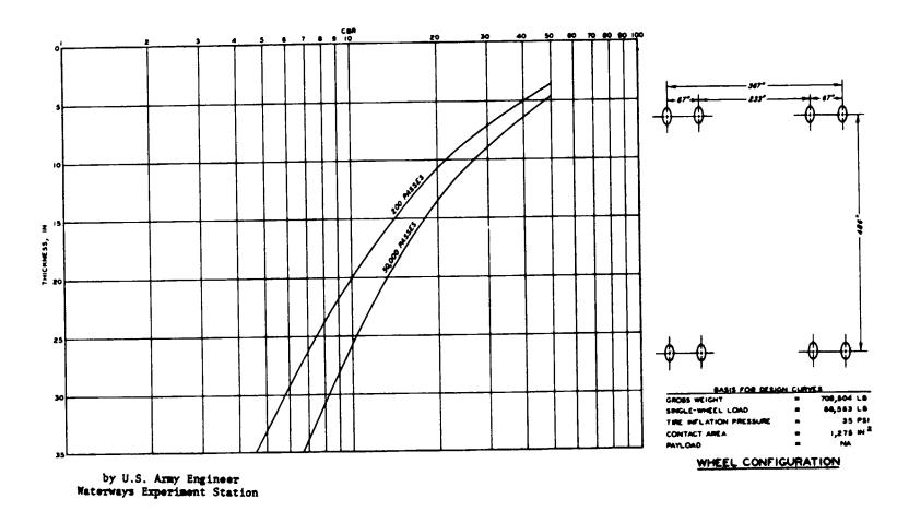
Figure B-22. Flexible Pavement Curves for LeTro Crane GC-500 (mobile gantry crane).
