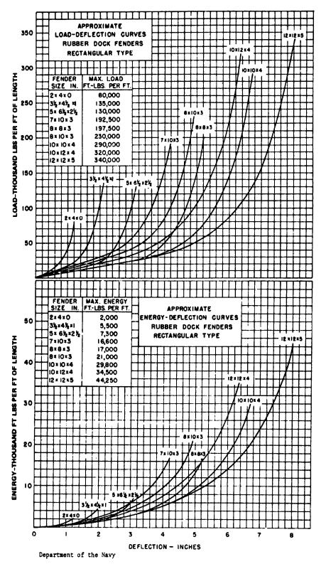
Figure 9-8. Load-Deflection and Energy-Absorption Characteristics (radially loaded rectangular rubber dock fenders).
