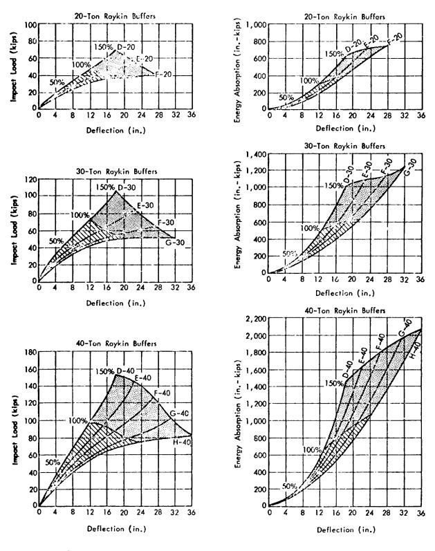
Figure 9-11. Load-deflection and energy-absorption characteristics of commercially available Raykin buffers.
