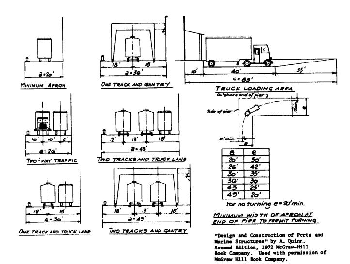
Figure 6-2. Various widths of apron for different operating conditions.
