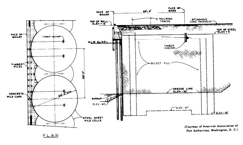
Figure 8-13. Solid fill-type wharf construction with circular steel sheet pile cells.
