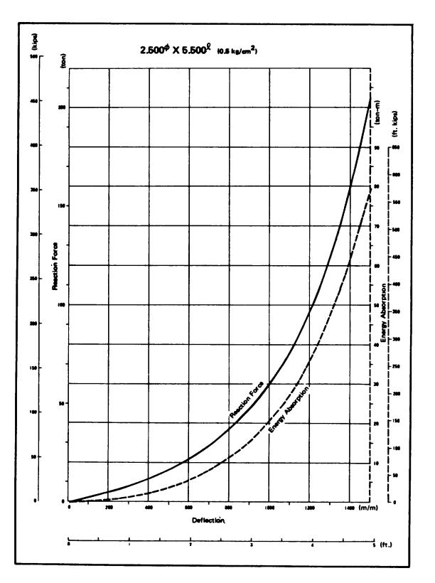
Figure 9-17. Yokohama Pneumatic Rubber Fender (this size used for berthing 5,000- to 20,000-ton ships)
