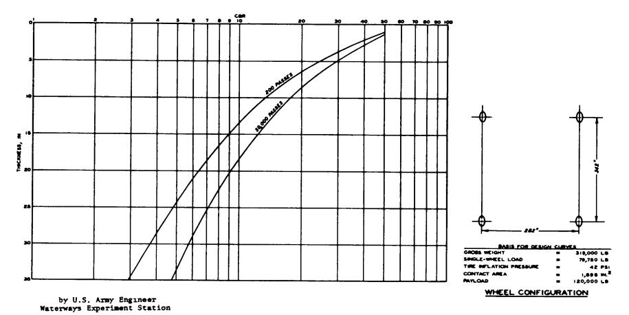
Figure B-13. Flexible Pavement Design Curves for LARCLX (amphibian).
