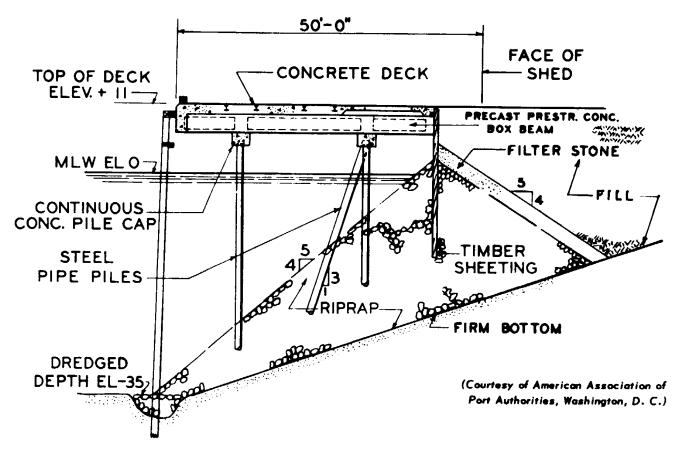
Figure 8-10. High-Level Open-Type Wharf Construction with Concrete Deck on Prestressed Concrete Beams-Steel Pipe Piles.
