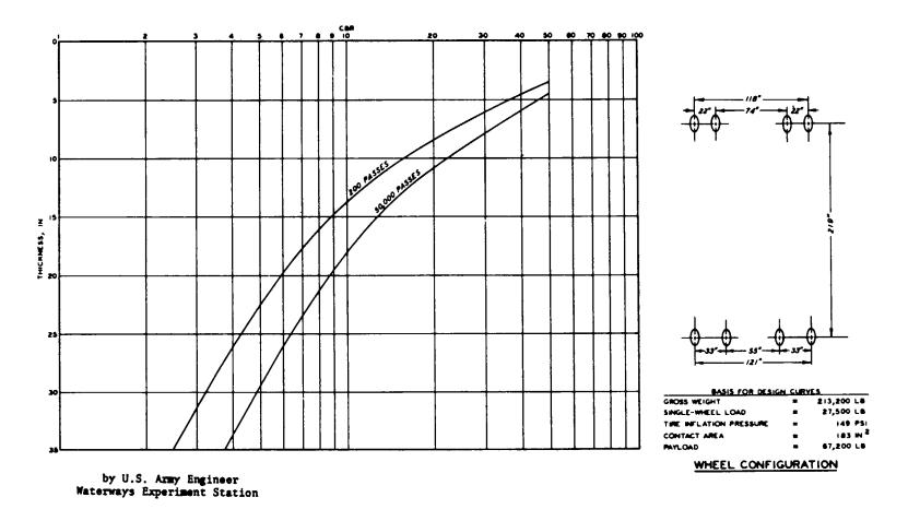
Figure B-19. Flexible Pavement Design Curves for Lancer 3500 (side-loading forklift).
