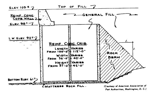
Figure 8-15. Solid fill-type wharf construction with reinforced concrete crib wharf.
