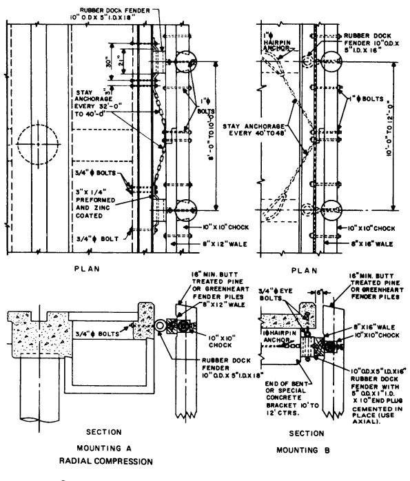
Figure 9-6. Resilient Fender System (rubber-in-compression).
