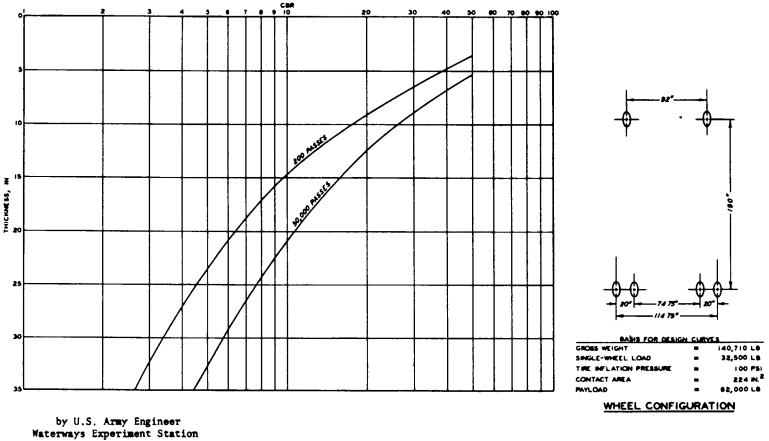
Figure B-17. Flexible Pavement Design Curves for Hyster H620B (front-loading forklift)
