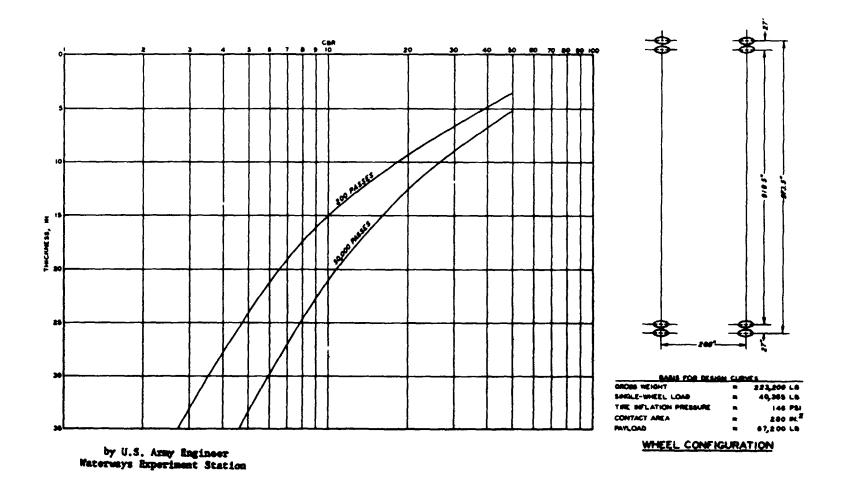
Figure B-20. Flexible Pavement Design Curves for Travelift CH 1150 (yard gantry).
