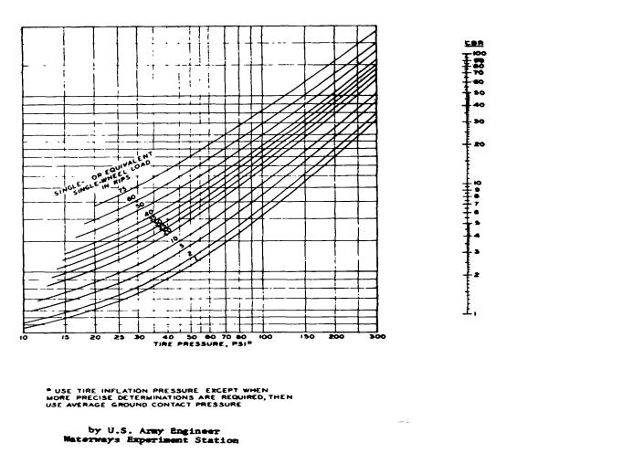
Figure B-12. CBR required for operation of aircraft on unsurfaced soil.
