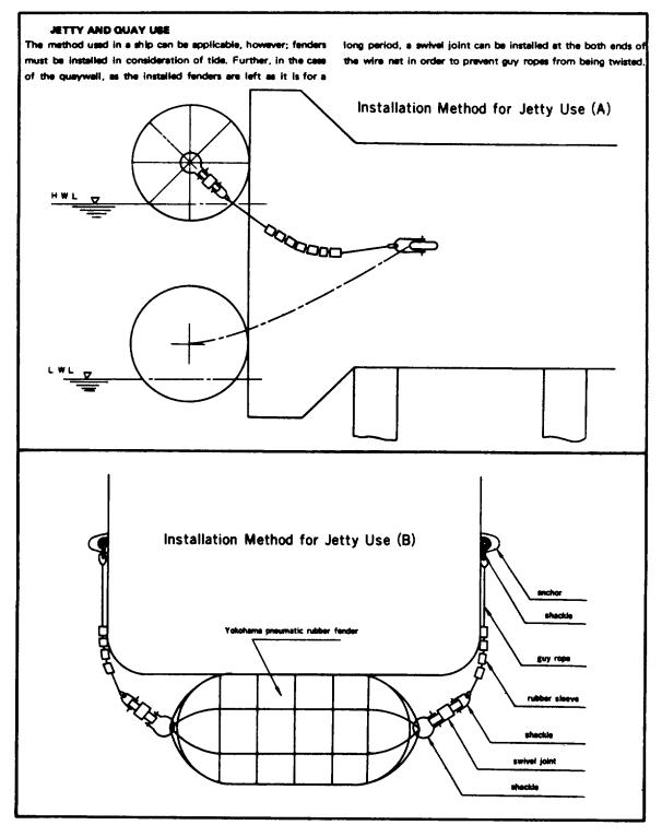
Figure 9-15. Yokohama Pneumatic Rubber Fenders (jetty and quay use).
