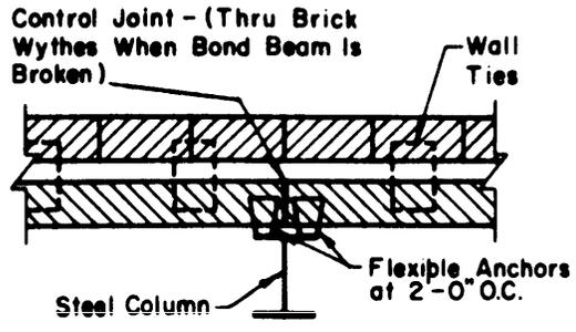
STEEL COLUMN-WITH CONTROL JOINT
