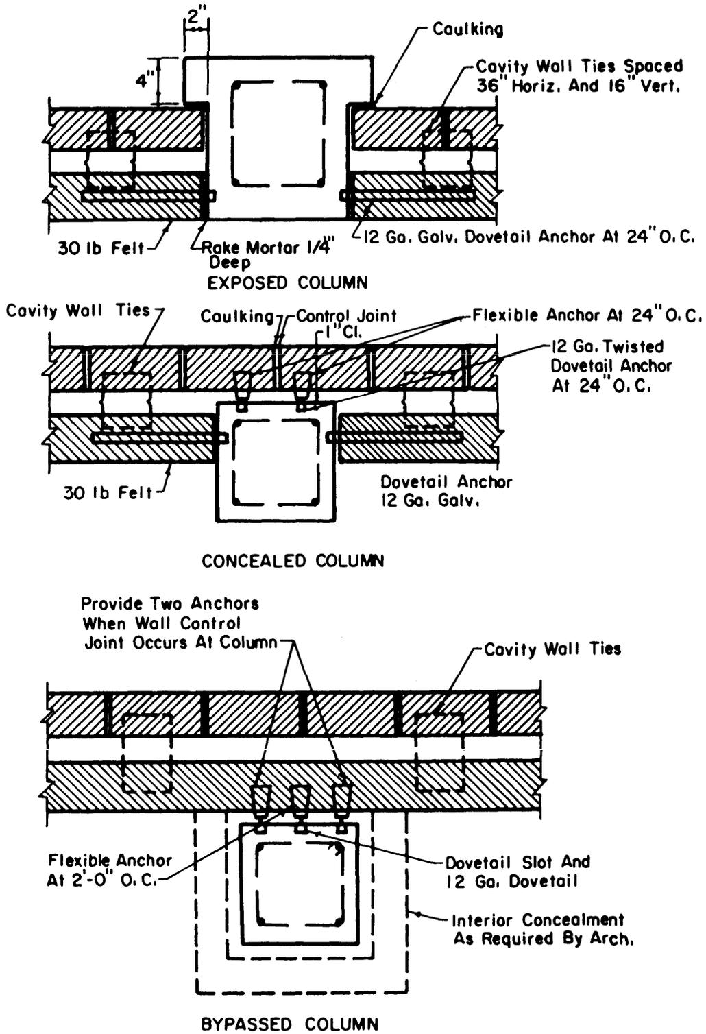
Note: Ties to column are required only when ties to beam are omitted.
