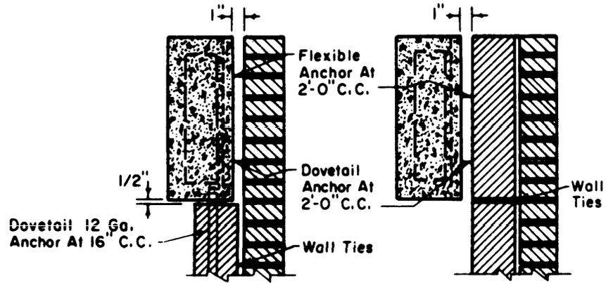
WALL ANCHORAGE TO CONCRETE BEAM
