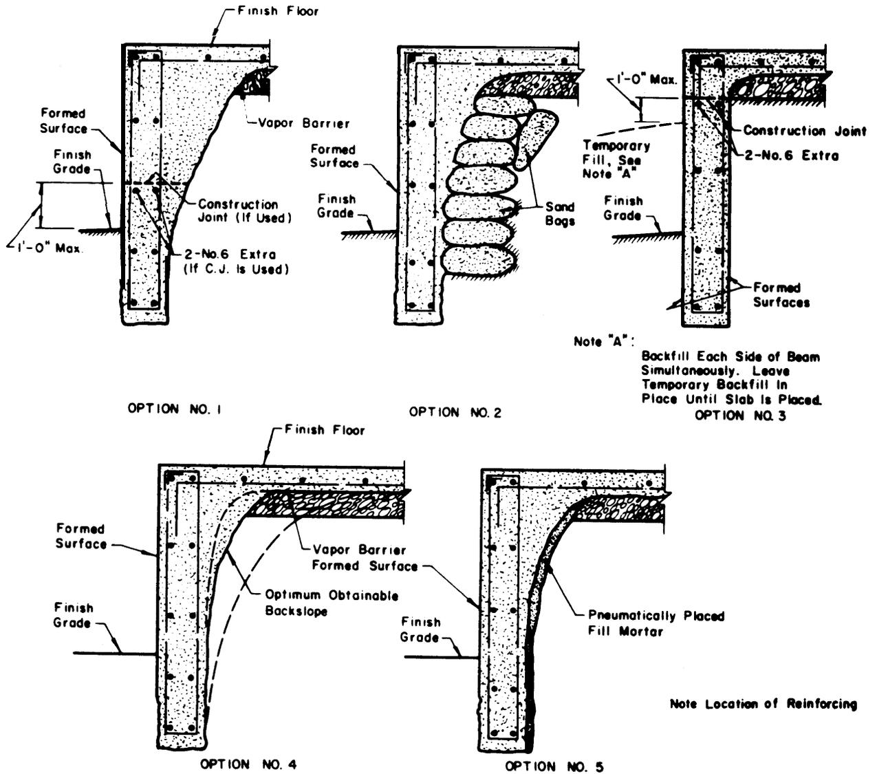
Figure C-10. Optional construction details of exterior beams (interior beam similar) for ribbed mat construction.
