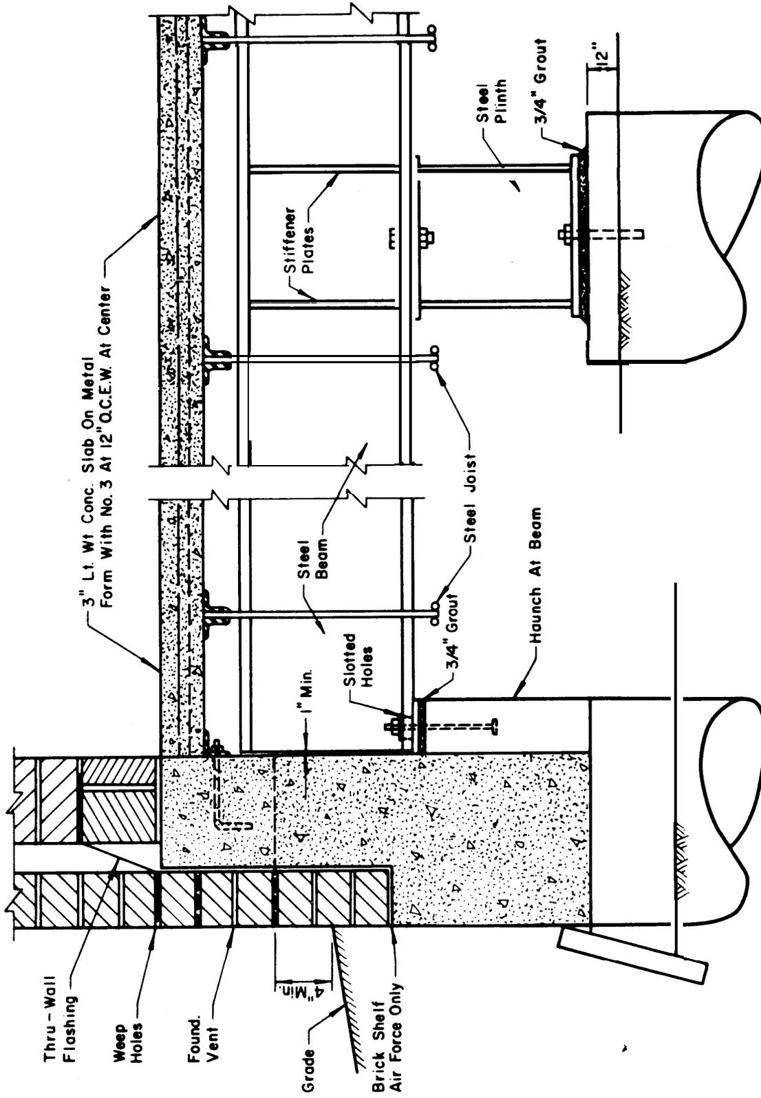
Figure C-7. Typical bar joist first floor framing.
