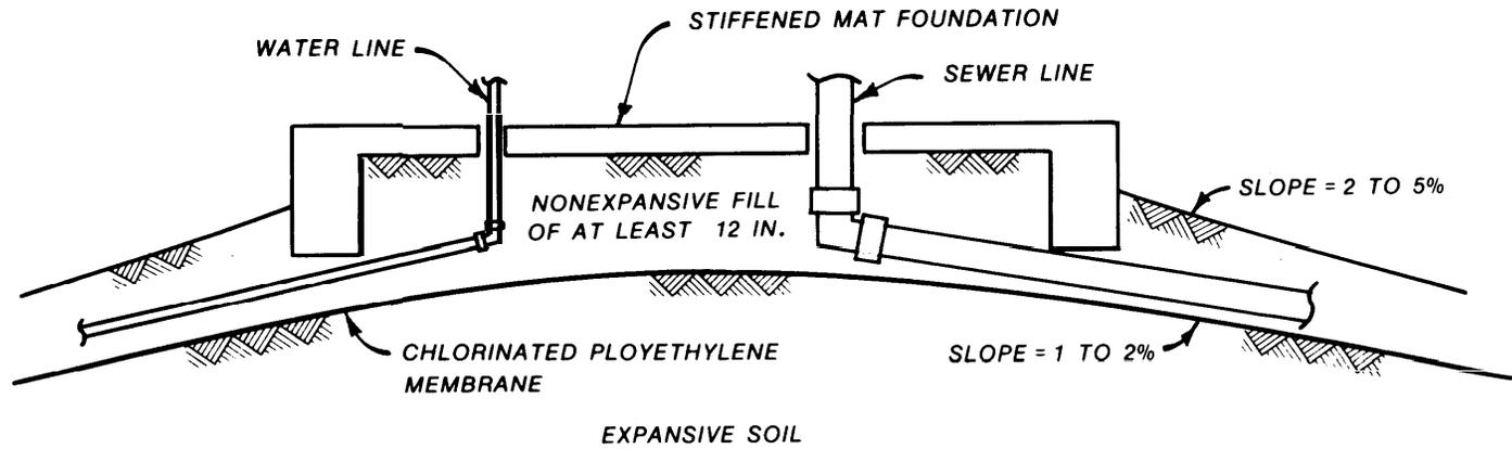
NOTE: POTENTIAL SOURCES OF WATER SHOULD BE LOCATED ABOVE THE MEMBRANE.
