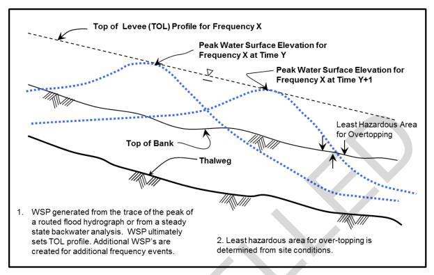
Figure 2. Top of levee (TOL) profiles
