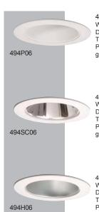
WhiteTrim Ring and White Reflector Die-cast trim ring and aluminum reflector Trim ring height of .160" at OD and .180" at ID Provides clearance for remodeler flange and gasket for AIR-TITE seal
