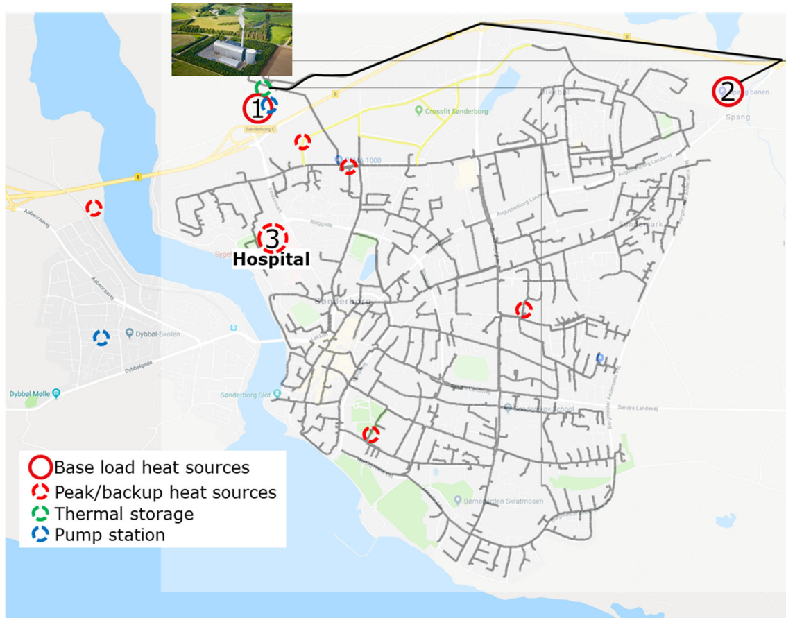
Figure 7-10. Sønderborg district heating system. The base load plant is a waste incineration CHP with a large thermal storage.
