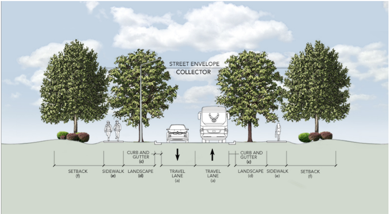
Travel Lane (a): 12' Median (b): N/A Curb and Gutter (c): 2' Landscape (d): 10' Sidewalk (e): 6' Setback (f): Min. 35' or per ATFP
