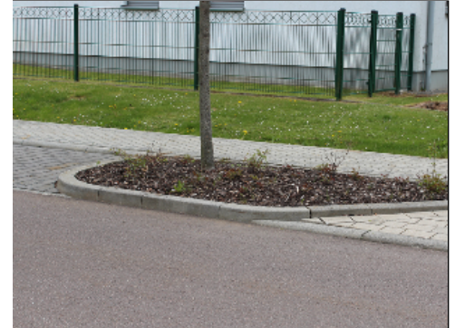
Buffering Median at Parallel Parking
