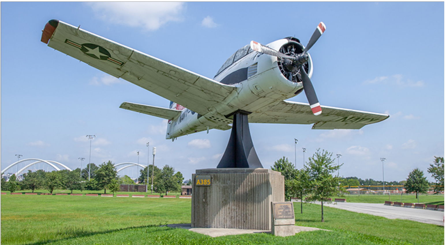
Dynamic Mounting of Aircraft with Steel Post and Concrete Base
