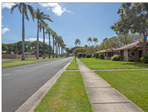
Detached Sidewalk with Grass Parkway
