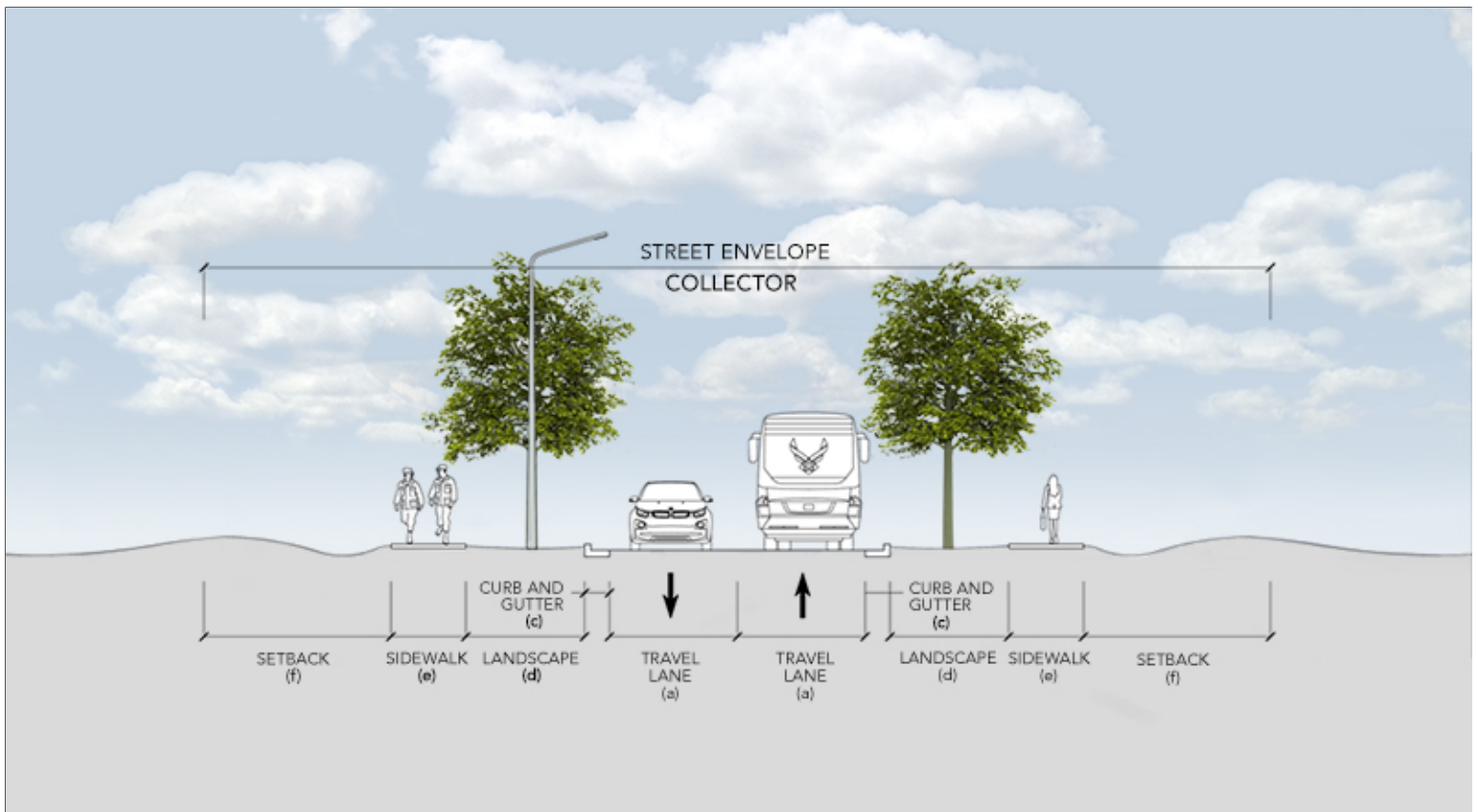
Travel Lane (a): 12' Median (b): N/A Curb and Gutter (c): 2' Landscape (d): 10' Sidewalk (e): 6' Setback (f): Min. 35' or per ATRP
