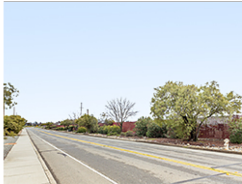
Attached Sidewalk on Single Side
