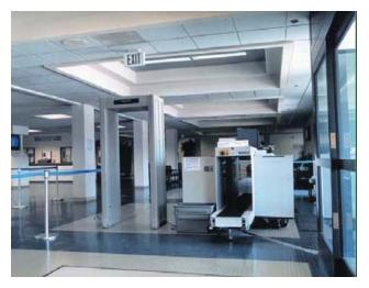
X-Ray and Magnetometer Equipment for Security Screening
