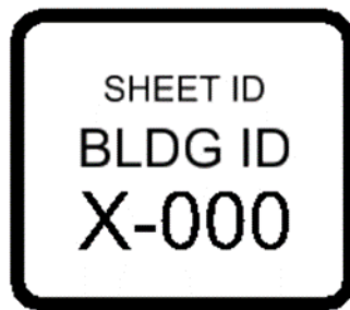
Figure 2-10. Sheet Identification block.
