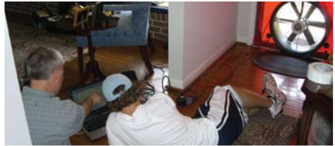
Figure 1. Initiating the Depressurization Test on attached laptop.
